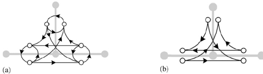
Figure 4: a) the complete pseudo-dual graph b) the restricted pseudo-dual graph (reproduced from Winter 2002)
