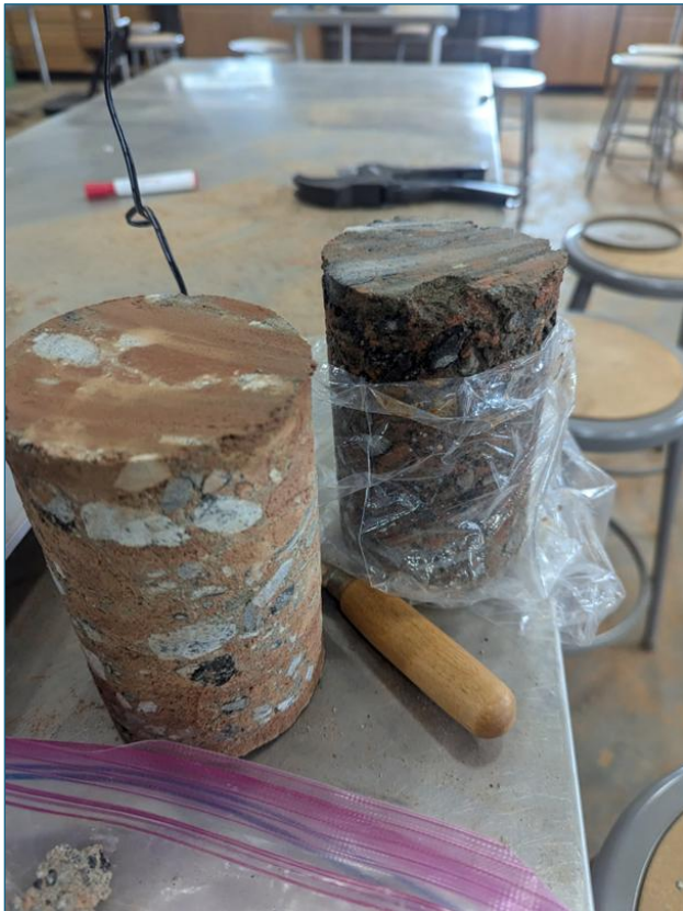
Figure 26. Photos. Collected core samples from the stabilized base.
