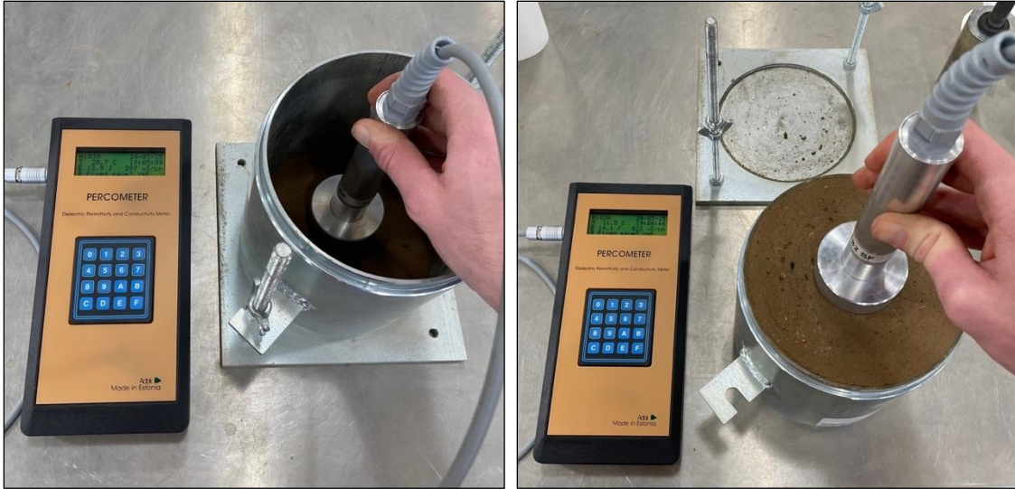
Figure 15. Photos. Percometer scanning top (left) and bottom (right) of samples.
