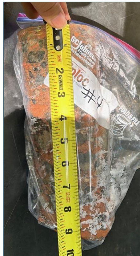
Figure 26. Photos. Collected core samples from the stabilized base.
