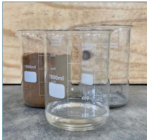
Figure 13. Photo. Soil-cement sample mixture (5.5 percent cement and 10 percent water).
