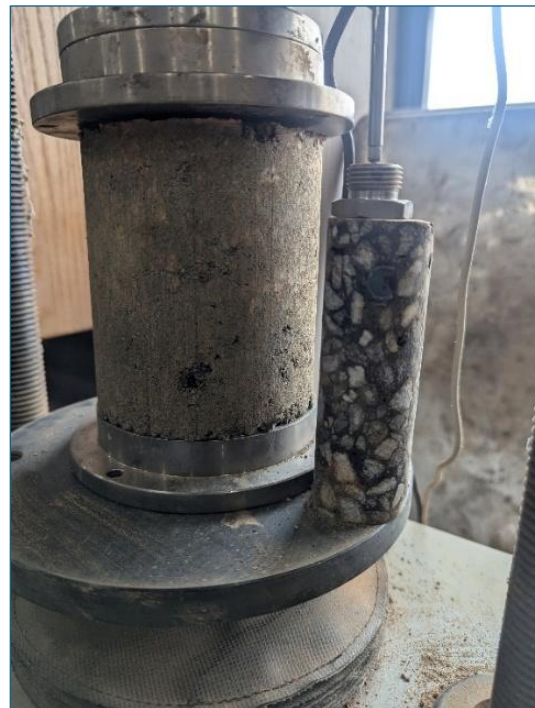
Figure 22. Photo. Crushing the FDR sample during the UCS test.
