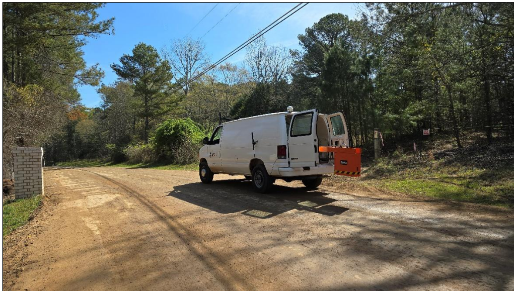
Figure 10. Photo. GPR van scanning the stabilized FDR base at Daniels Bridge Road.
