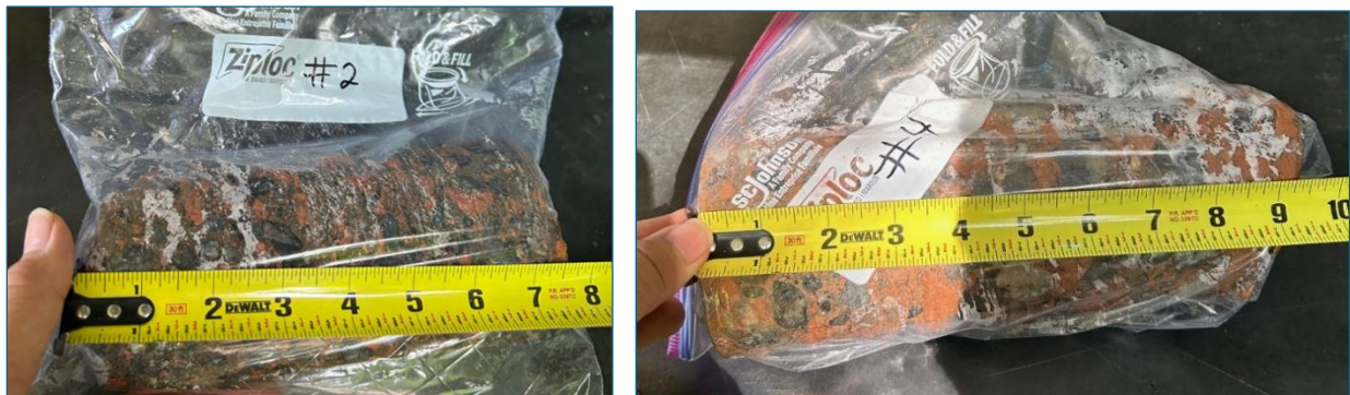
Figure 56. Photos. Field core samples confirming the as-built layer thickness.
