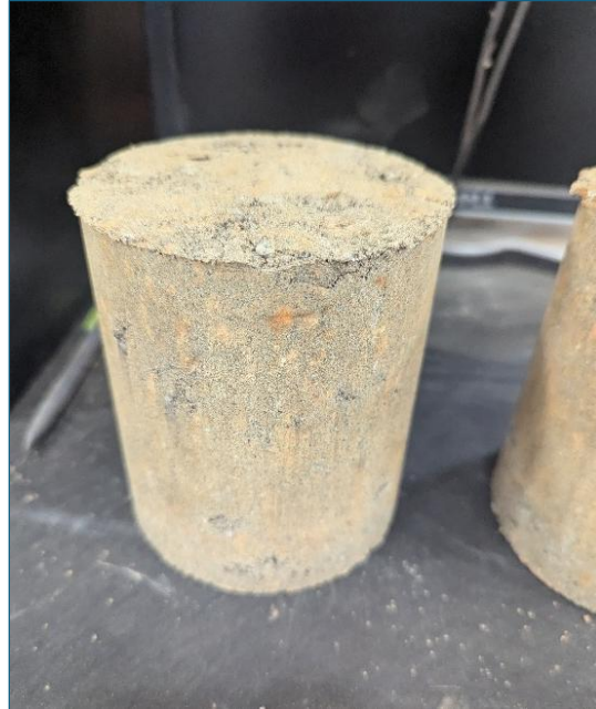
Figure 21. Photo. Molded FDR cement sample.
