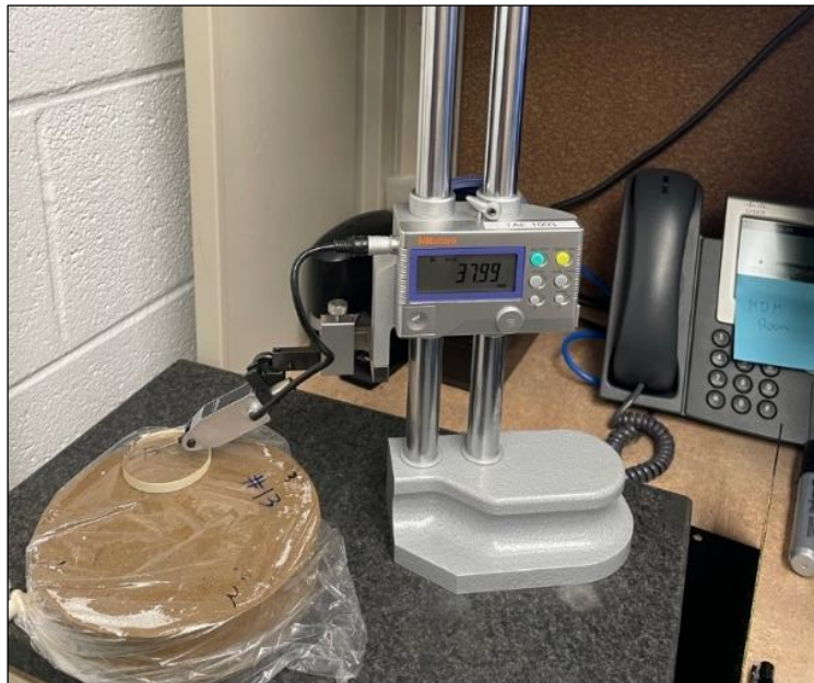
Figure 17. Photo. MDM sample thickness measurement.
