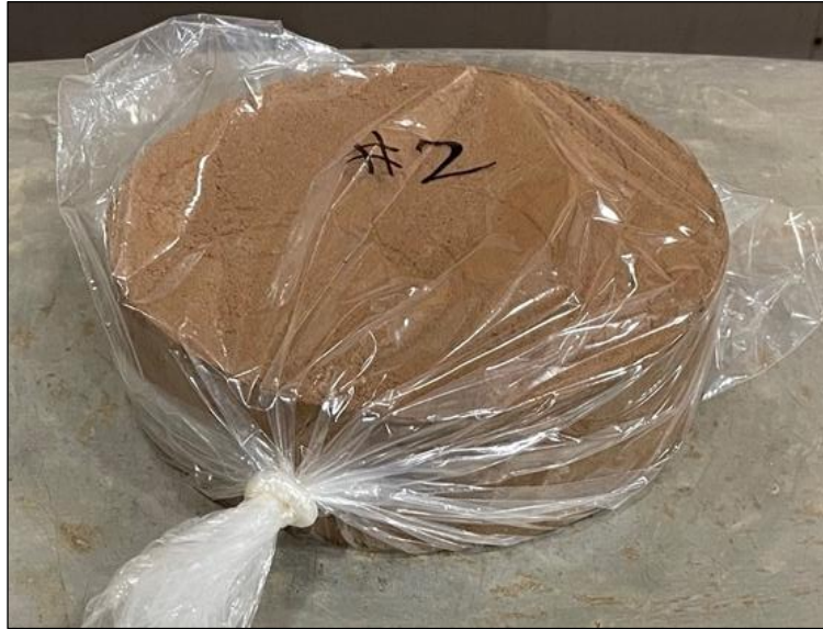
Figure 16. Photo. Soil-cement MDM sample.
