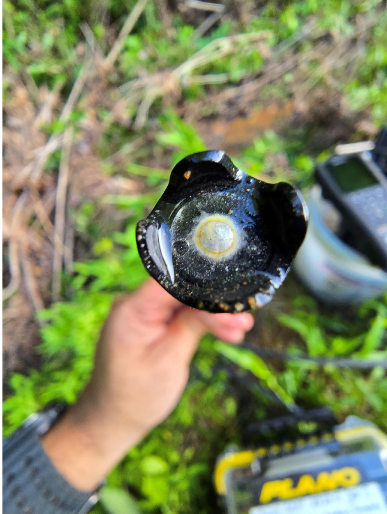
Figure 93. Photo. DFRobot® DO Sensor Cap Degraded by Fouling.
