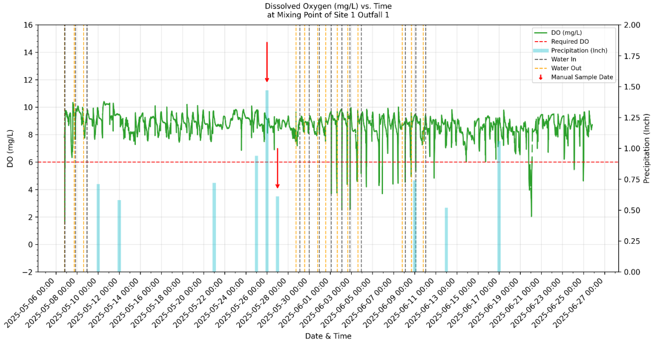
Figure 55. Chart. HOBO® DO vs Time plot with USGS daily Precipitation data ( \geq 0.5 inch) at Mixing point of Outfall 1 from 2 nd Quarter of 2025
