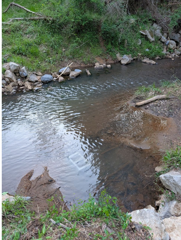
Figure 17. Photo. Initial deployed placement of instream sensor concrete (CC) block at Site 2
