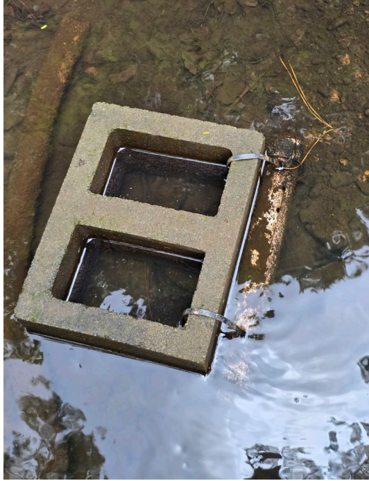
Figure 18. Photo. HOBOTM Data logger inside protective housing, anchored with CC block at Site 2 Outfall 1.
