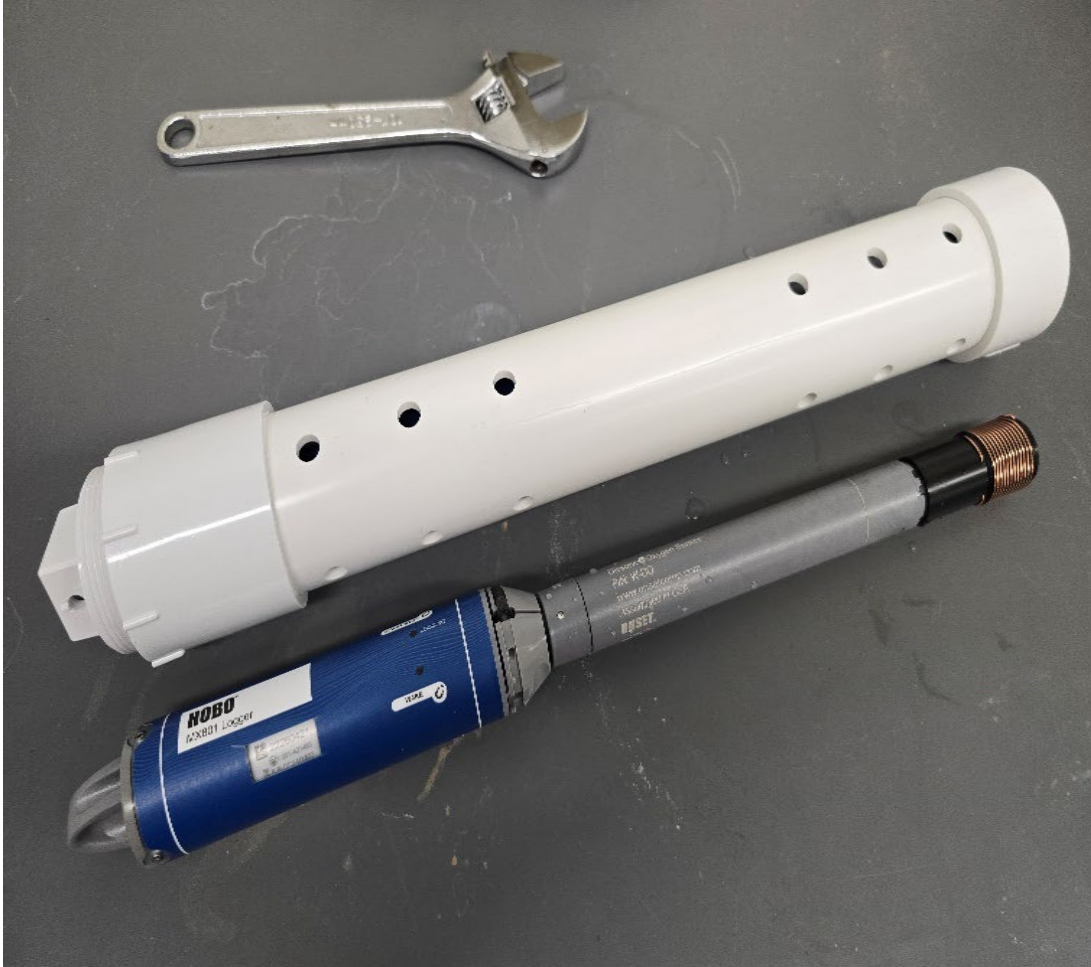
Figure 10. Photo. HOBO® Data Logger with DO/Temperature Sensor Attached and PVC Protective Housing
