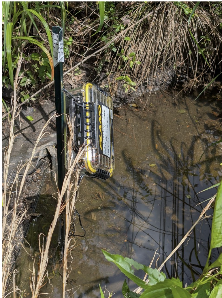
Figure 12. Photo. Deployed ESP32-based Remote Sensor System at Site 1 Outfall 2
