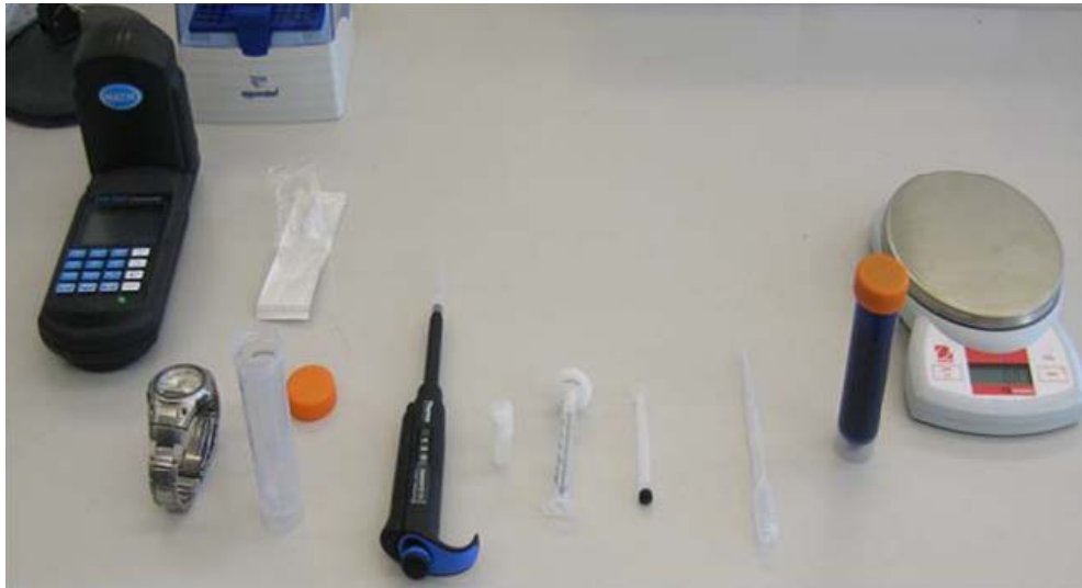
Figure B-1 Methylene Blue Test apparatus [139]
