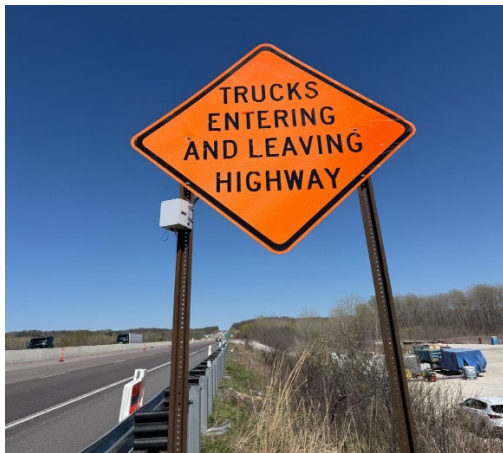
Figure 1: Example of sensor mounted on existing sign at I-70 Rocheport.
