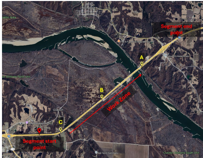
Figure 5-11. Aerial showing HERE segment and speed sensors for I-70 Rocheport.
