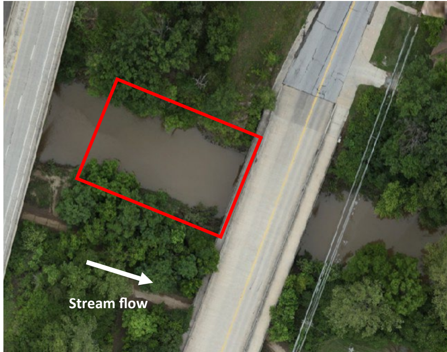
Figure 4.15 UAV orthoimage showing the selected analysis region for upstream surface velocity estimation. The red box indicates the area for PIV analysis, with flow direction shown by the white arrow.
