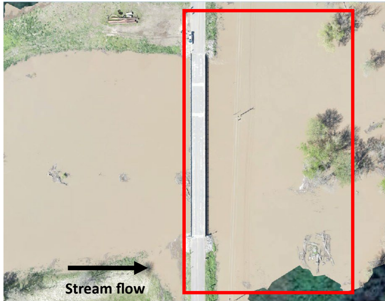
Figure 4.6 UAV orthoimage showing the selected analysis region for downstream surface velocity estimation. The red box indicates the area for PIV analysis.
