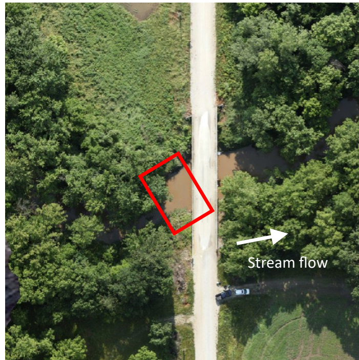
Figure 4.24 UAV orthoimage showing the selected analysis region for upstream surface velocity estimation for Moniteau Creek. The red box indicates the area for PIV analysis, with flow direction shown by the white arrow.
