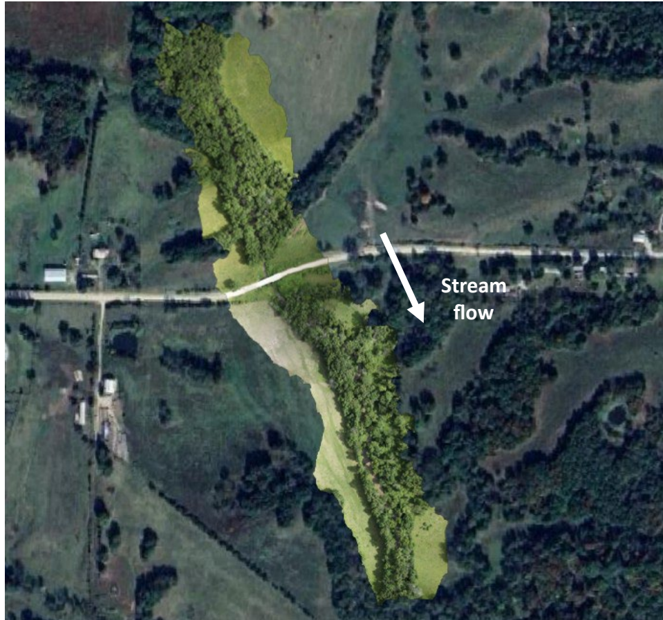
Figure 4.28 UAV-derived orthophoto of the Long Branch Creek survey area captured with the DJI P1 camera.
