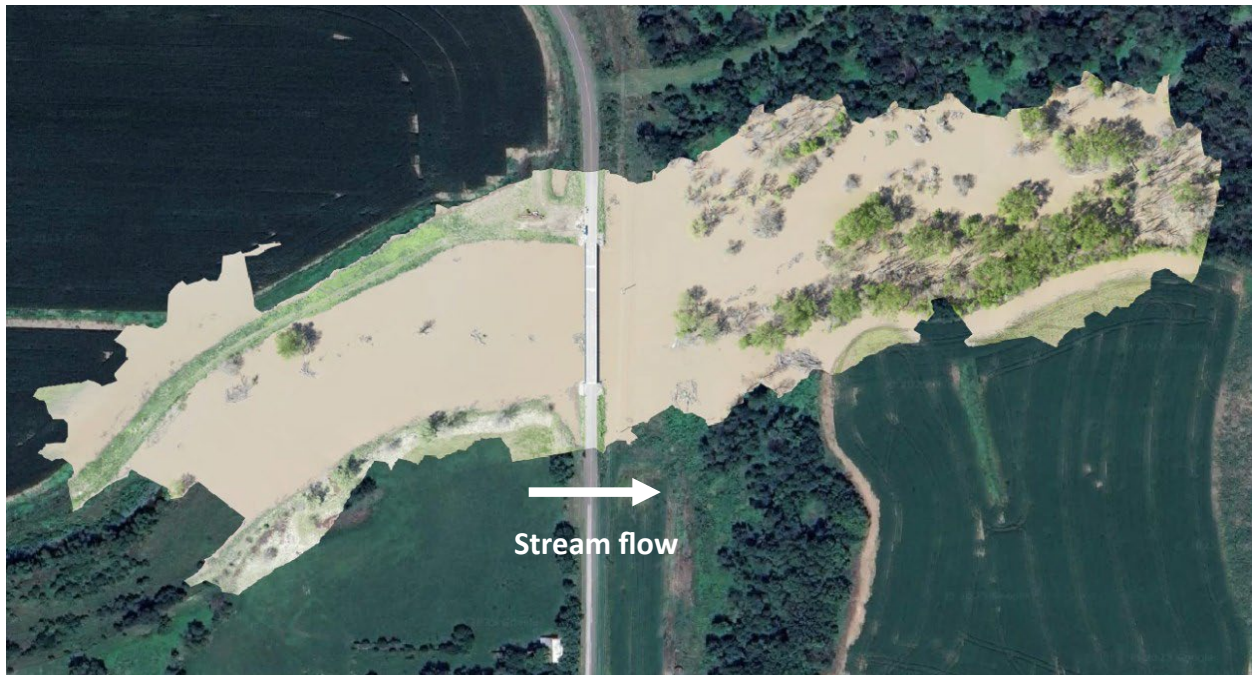
Figure 4.1 UAV-derived orthophoto of the Petite Saline Creek survey area. The orthophoto, generated from high-resolution imagery collected by the DJI M350–P1 system.
