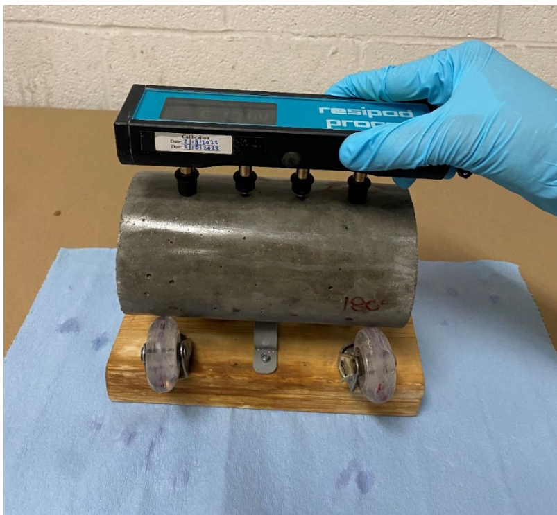
Figure 6. Concrete sample surface resistivity measured according to AASHTO T 358, figure by Raid Alrashidi used with permission
