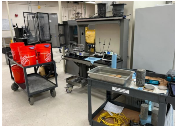
Figure 42. Resistivity testing setup
