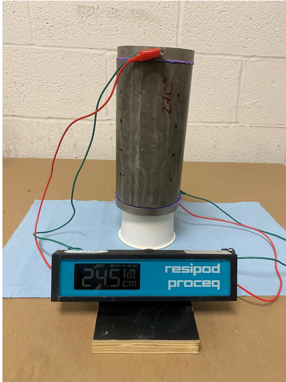
Figure 5. Concrete sample uniaxial resistivity measured according to AASHTO TP 119, figure by Raid Alrashidi used with permission
