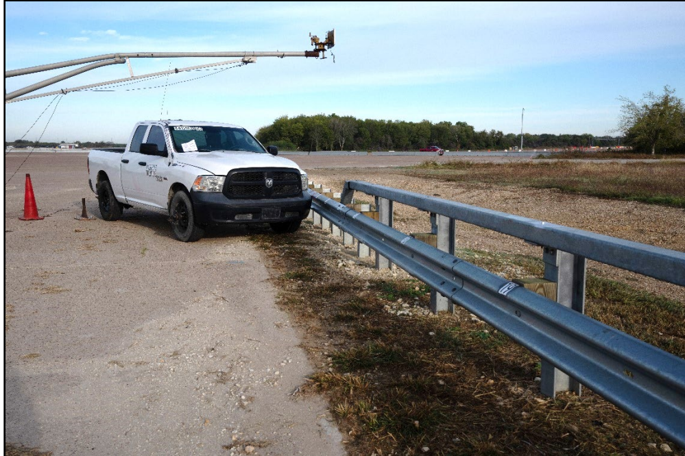
Figure 7.1. Transition and Test Vehicle Geometrics for Test 441203-01-2.
