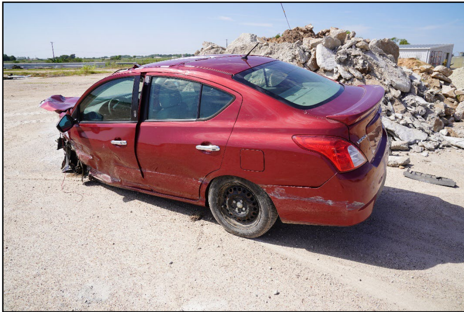
Figure 6.8. Rear Impact Side of Test Vehicle after Test 441203-01-1.
