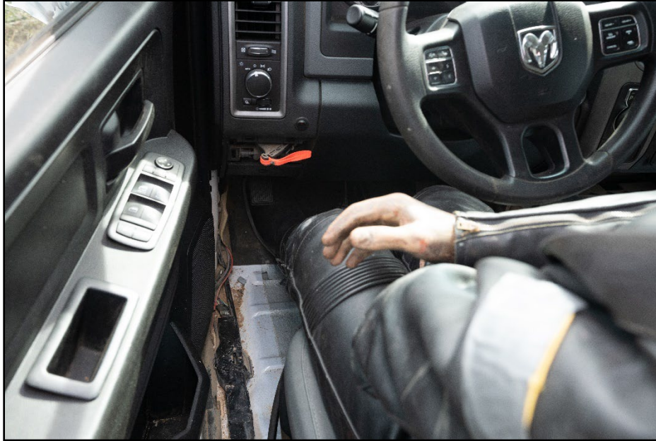
Figure 7.10. Interior of Test Vehicle on Impact Side after Test 441203-01-2.
