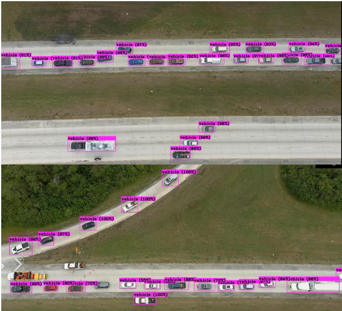
Figure 5. Detected vehicles after model retraining.
