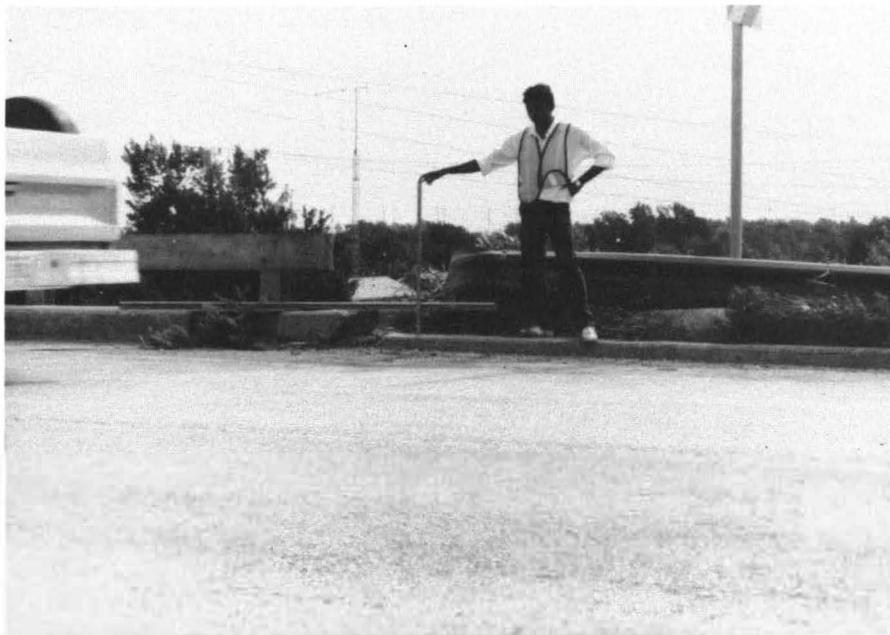
Fig. 4. Settlement estimate of bridge approach from the differential settlement of the curb.
