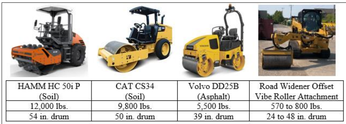
Figure 22. Example of Compactors for Narrow Widening ( https://www.wirtgen-group.com/ , https://www.cat.com/ , https://www.volvoce.com/ ).
