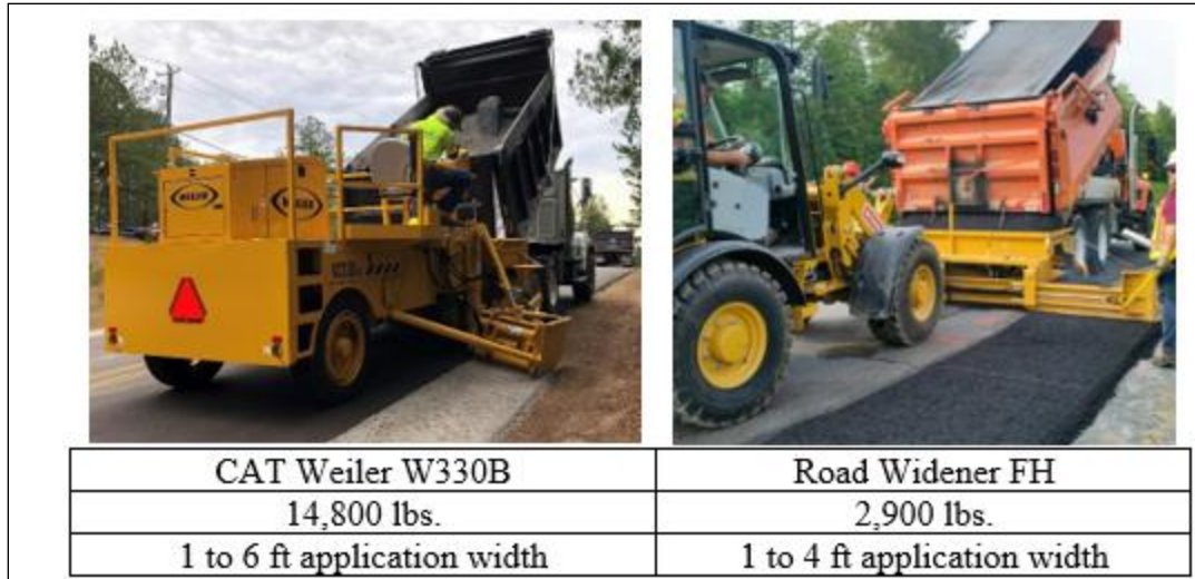
Figure 21. Roadway Wideners ( https://www.weilerproducts.com/ , https://www.roadwidenerllc.com/ ).
