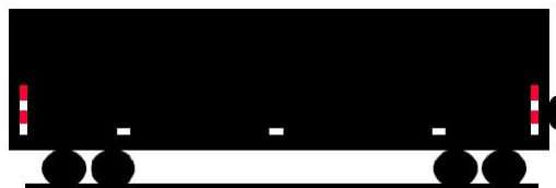
Figure 8. Freight car reflectorization pattern used in the in-service revenue test conducted by Carroll, et al. (1999).
