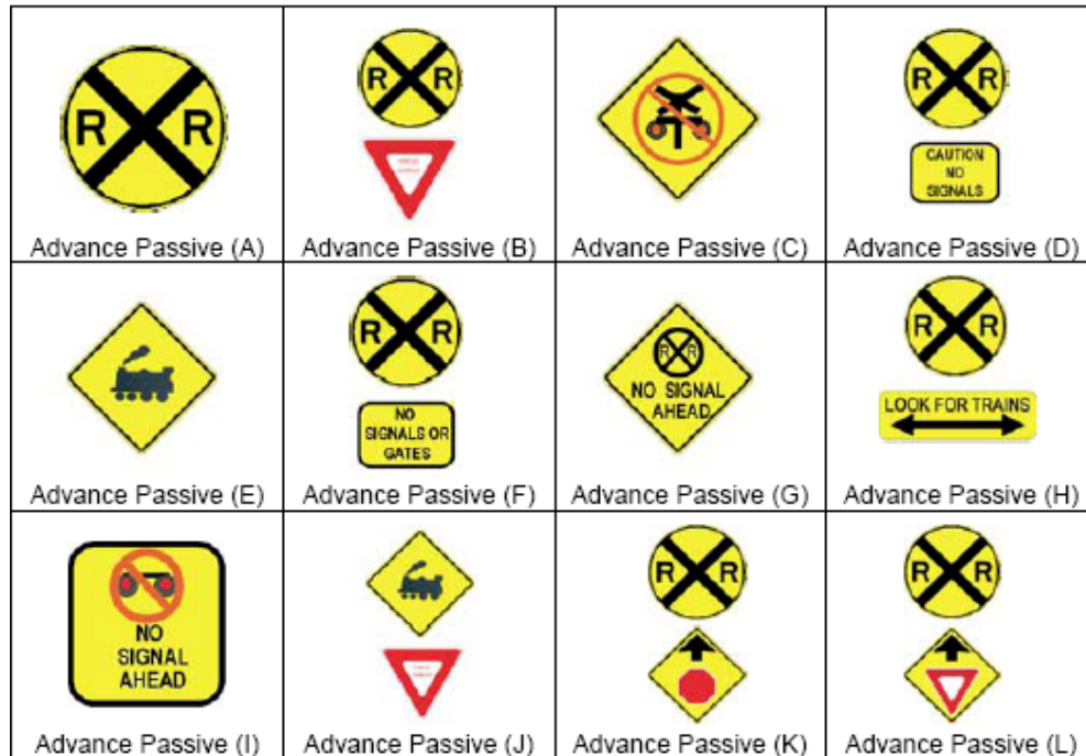
Figure 5. Advance warning signs for passive crossings.
