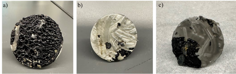
Figure 4.12 Dollies after the POTS test: (a) Binder-Aggregate; (b) Binder-LDPE-Aggregate; (c) Binder-PP-Aggregate.
