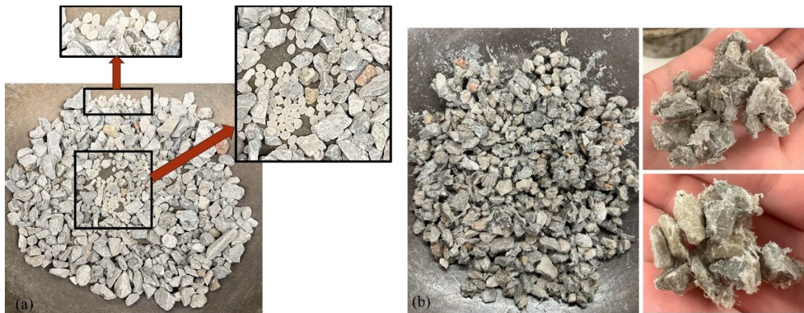
Figure 4.4 Aggregates and PP mixed at: a) 156°C; b) 194°C.
