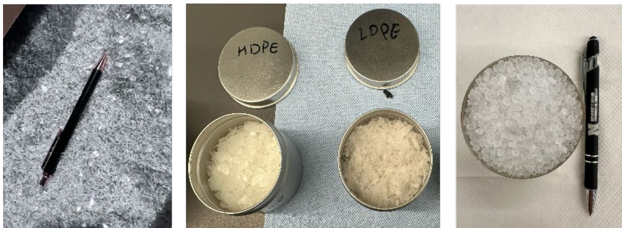
Figure 3.2 WP samples used in this study (from left to right): PET, HDPE, LDPE, PP.
