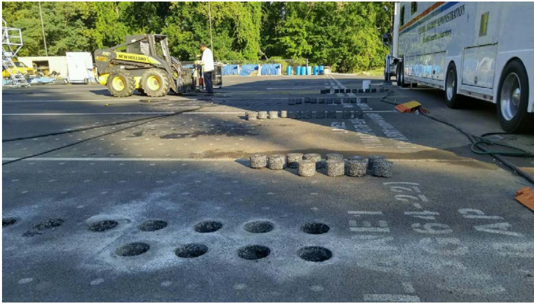
Figure 26 – Field Cores Recovered from FHWA ALF for Asphalt Mixture and Binder Testing
