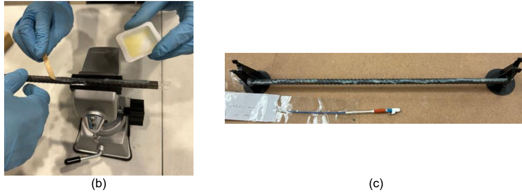
Figure 4. Sensor embedding on rebar: (a) The schematic of the experimental setup of the smart composite reinforced concrete system. (b) applying epoxy on fiber optic sensor and rebar; (c) rebar after applying epoxy and tape.
