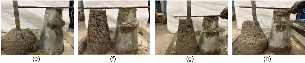
Figure 1. Slump test results (a) 0.2% fiber with 87 mL/kg water; (b) 0.2% fiber with 100 mL/kg water; (c) 0.4% fiber with 87 mL/kg water; (d) 0.4% fiber with 100 mL/kg water; (e) 0.4% fiber with 113 mL/kg water; (f) 0.6% fiber with 87 mL/kg water; (g) 0.6% fiber with 100 mL/kg water; (h) 0.6% fiber with 113 mL/kg water.
