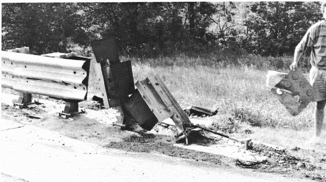
FIGURE 2.7 Sentre impact on Oklahoma turnpike
