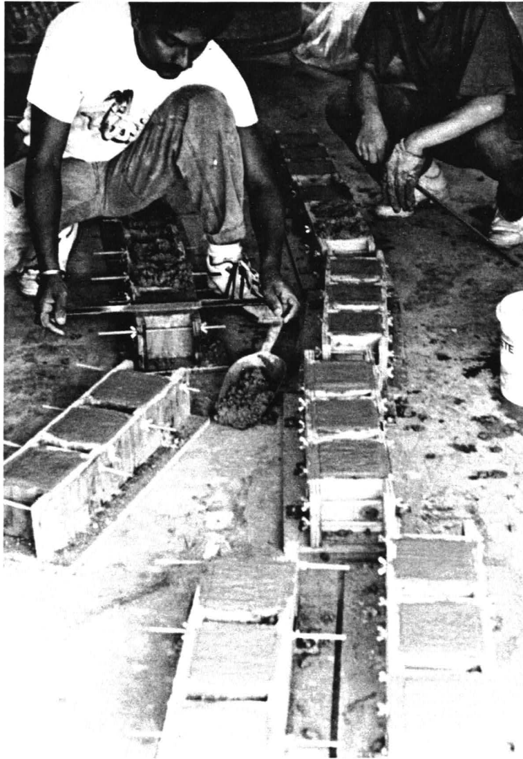
Fig. 3.6 Specimen Casting, NCHRP 244 Cubes
