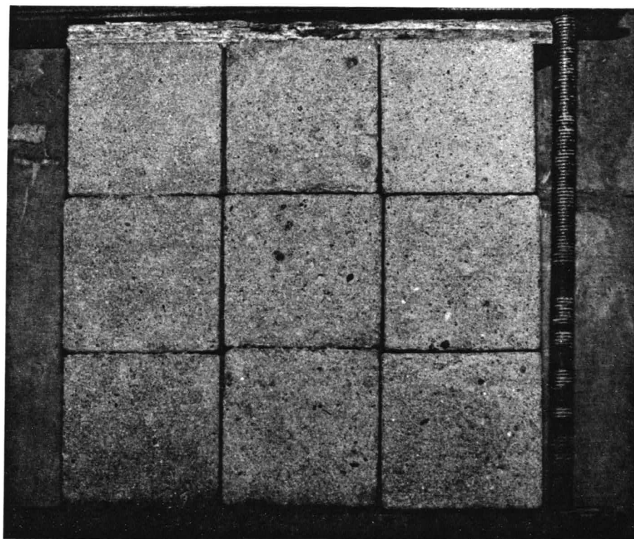
Fig. 3.10 Phase III Cubes After Shot-Blasting
