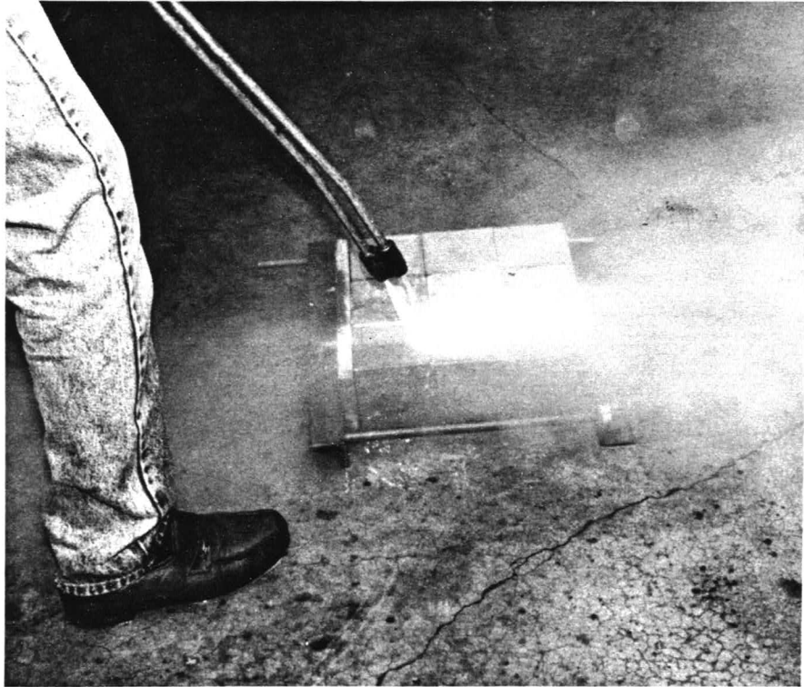
Fig. 3.11 High Pressure Water Washing, Phase III Cubes
