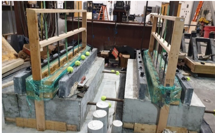
Figure 2.10: Pullout Specimens cast on Base Slabs 2 and 3
