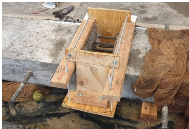
Figure 2.21: Formwork for Casting UHPC Strip for Beam-Splice Specimen
