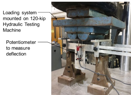
Figure 2.8: Flexure test setup
