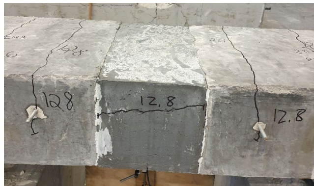
Figure 3.7: Splitting Crack on the Side of UHPC Strip in Beam-Splice Specimen
