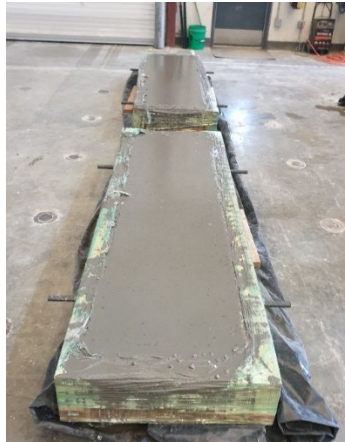
Figure 2.19: Beam-Splice Specimen Side Panels
