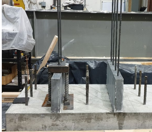
Figure 2.9: Pullout Specimens cast on Base Slab 1
