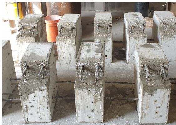
Figure 2.14: Base Blocks for Beam-End Specimens
