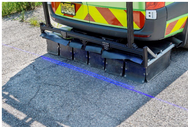
Figure 57 High Speed Sounding (Chain Dragging) [40]
