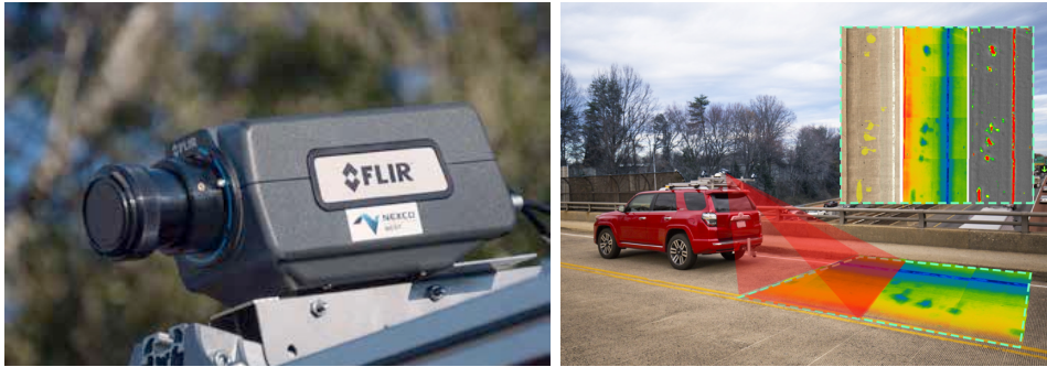
Figure 49 FLIR A6701sc Camera [43] and Deck Top Scanning System (DTSS) Include Infrared Thermography (IRT) [28] [44]
