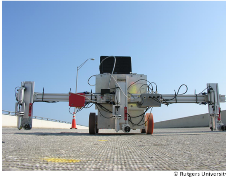
Figure 14 Impact Echo Equipment [39]
