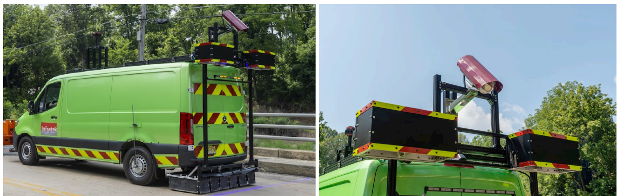
Figure 48 High Speed (HS) System Include Infrared Thermography (IRT) [40]
