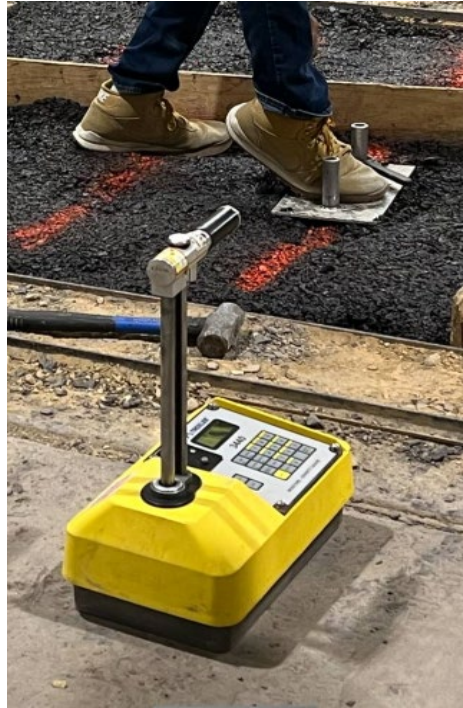
Figure 31 Nuclear Moisture-Density Gauge used in this study.
