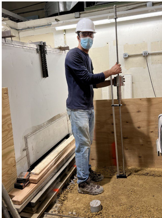
Figure 33. The DCP used in this study.
