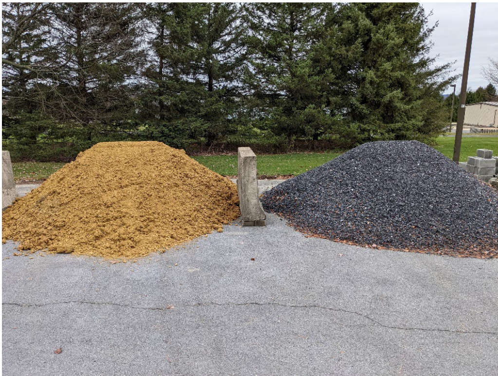
Figure 23: 2RC (left) and 2A (right) stockpiles at CITEL utilized in this study.
