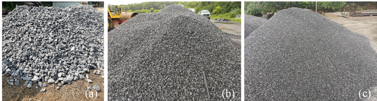
Figure 4-2. Aggregates used in field tests: (a) AASHTO #1; (b) AASHTO #57; (c) AASHTO #8.
