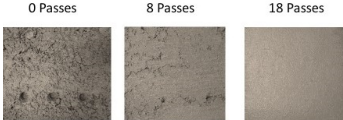
Figure 4-14: Mixture with poor finishability of mixture 52 with high amounts of #8.
