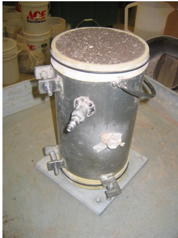
Figure 3-13 Compacted Resilient Modulus Specimen of Aggregate Base
