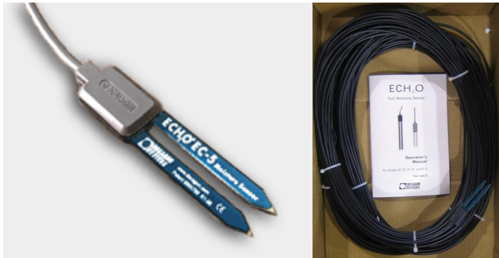
Figure 3-21 ECH2O EC-5 Moisture Probe
