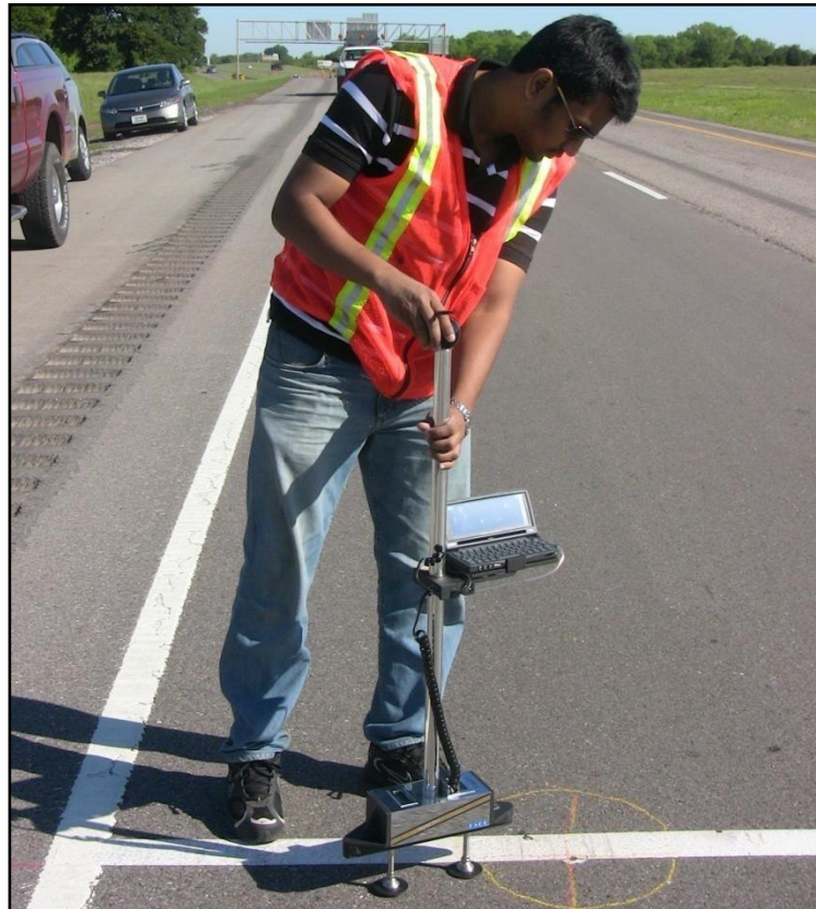
Figure 4-19 Data Collection with Face Dipstick®
