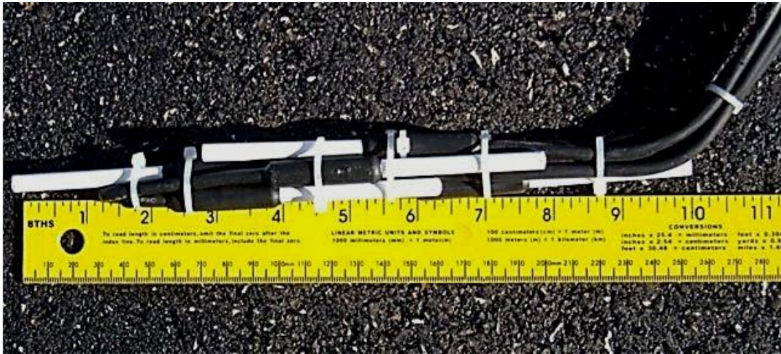
Figure 3-20 Thermistor Bundle for Measuring Pavement Temperature
