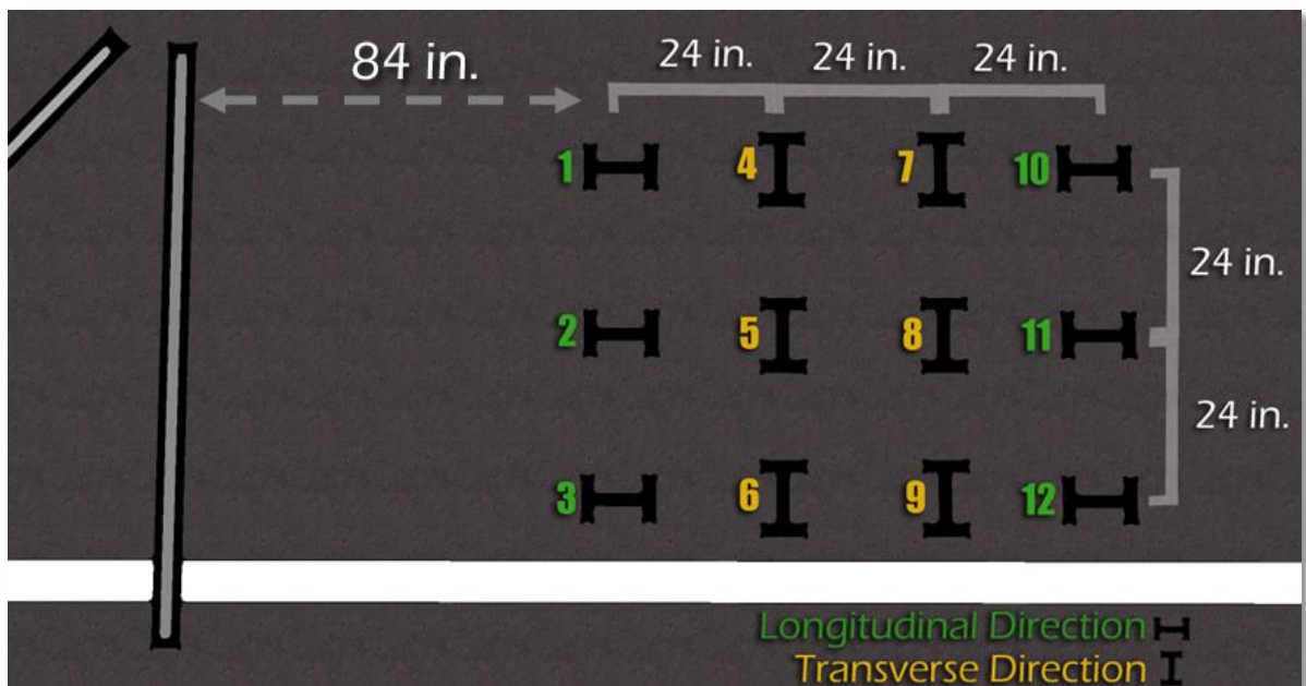
Figure 3-35 Layout of Strain Gauges
