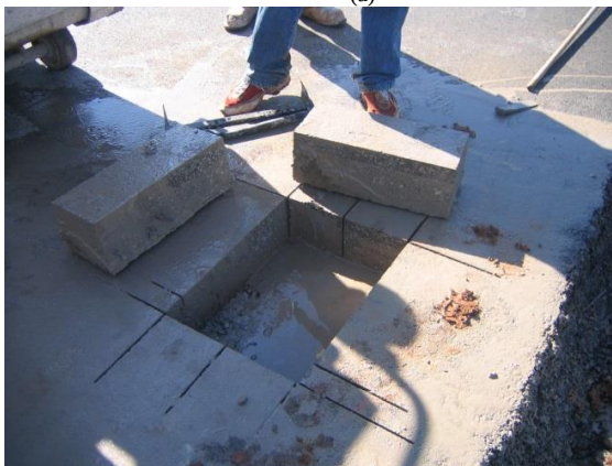
(c) (d) Figure 3-73 Extraction of Block Samples
