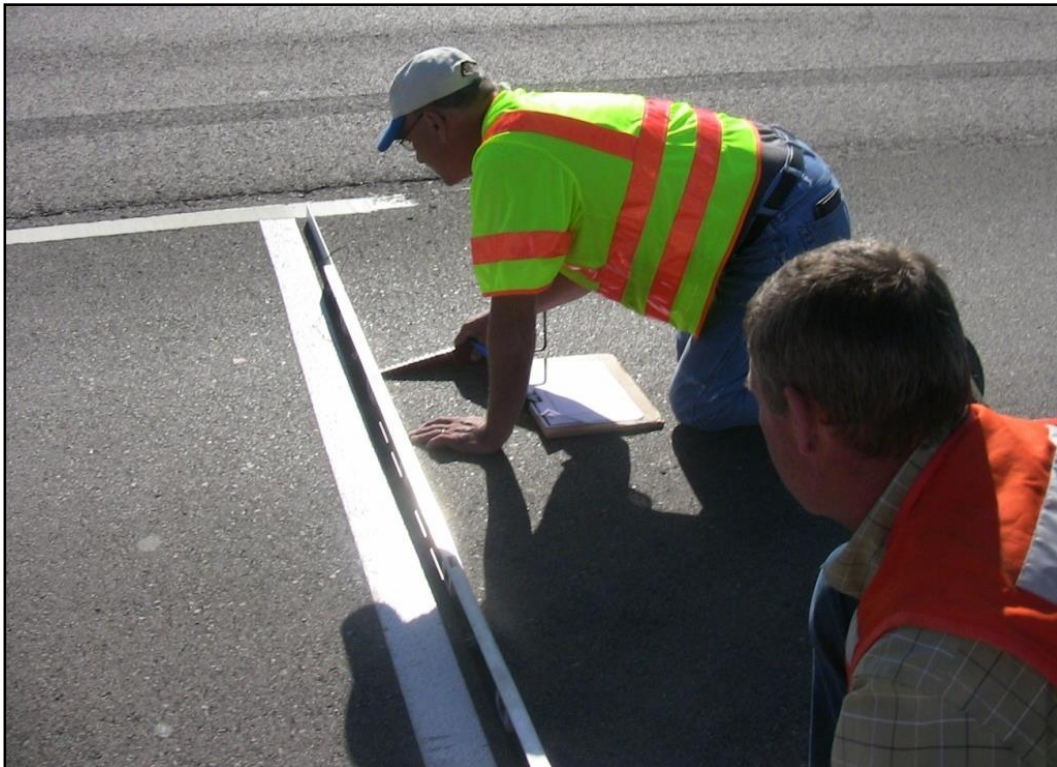
Figure 4-16 Rut Measurements with Straight Edge/Rut Gauge Combination
