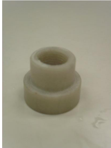
Figure 52: Ceramic Collar (P2) Suggested By Auburn University
