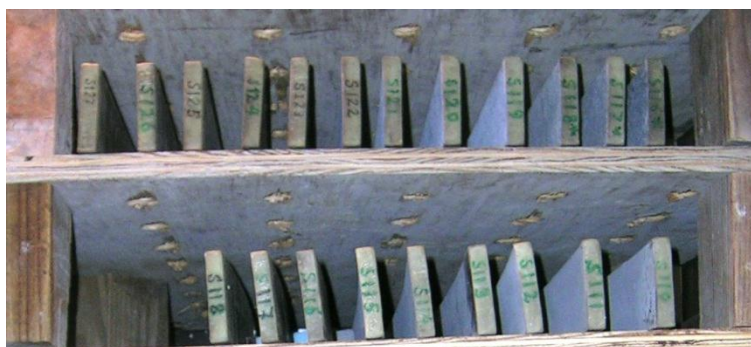
Figure 24: The Specimens Covered With Curing Compounds And Stored In The Chamber Room
