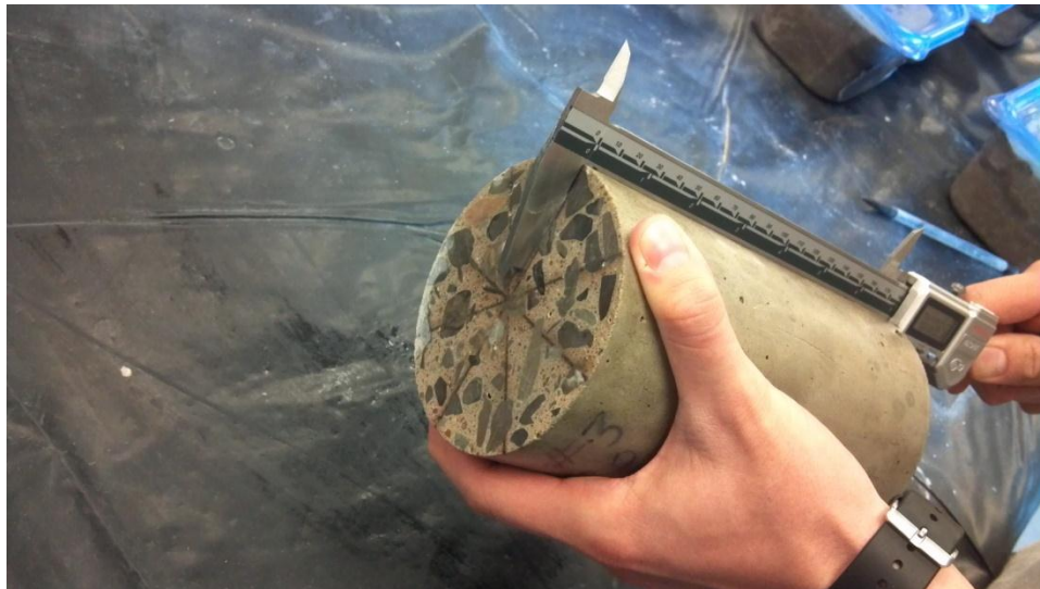
Figure 62: CTE Cylinder During Measurement With Alignment Markings
