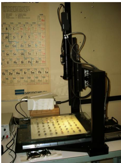
Figure 3-14 AIMS Sample Layout for: a) Coarse Aggregates, b) Fine Aggregates.
