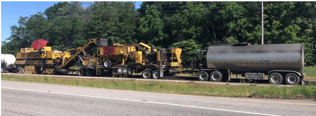
Figure 8. Multi-Unit Cold In-Place Recycling Train
