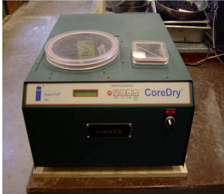
Figure 12 OSU's CoreDry™ apparatus.
