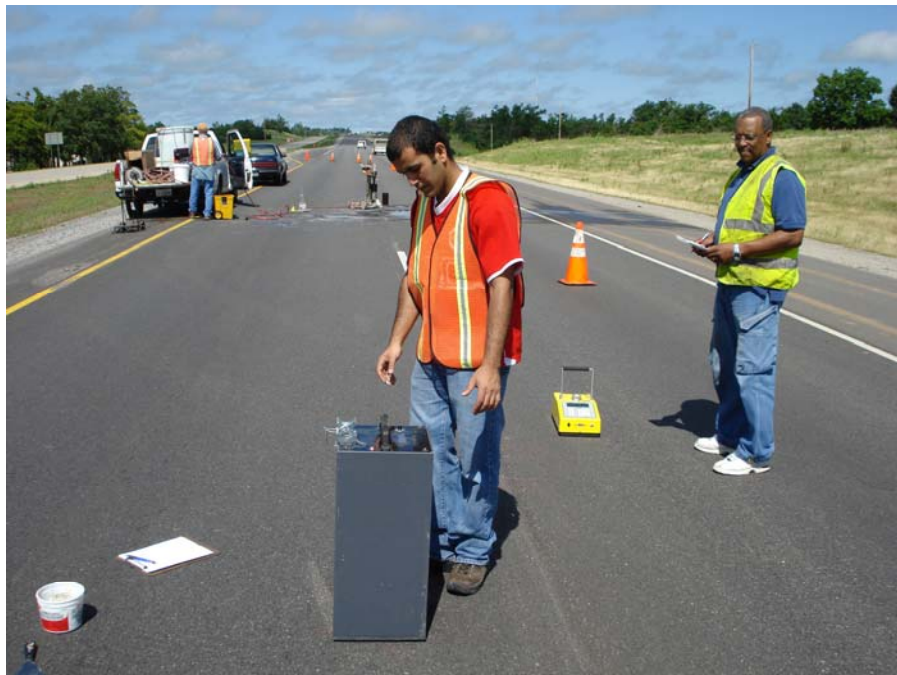
Figure 8 Measuring field permeability with the Romus air permeameter.
