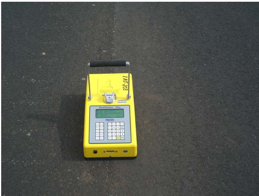
Figure 7 Electromagnetic gauge used for in-place density testing.
