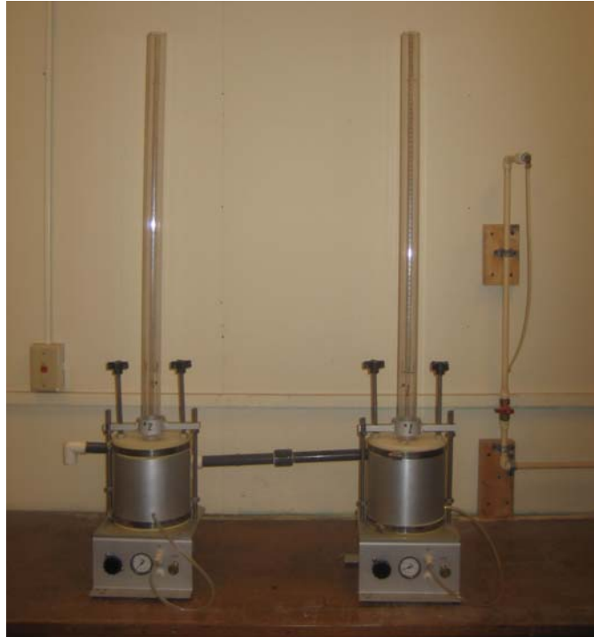
Figure 1 OSU's laboratory permeameters.
