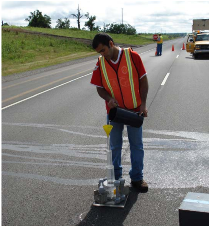
Figure 10 Measuring field permeability with NCAT permeameter.
