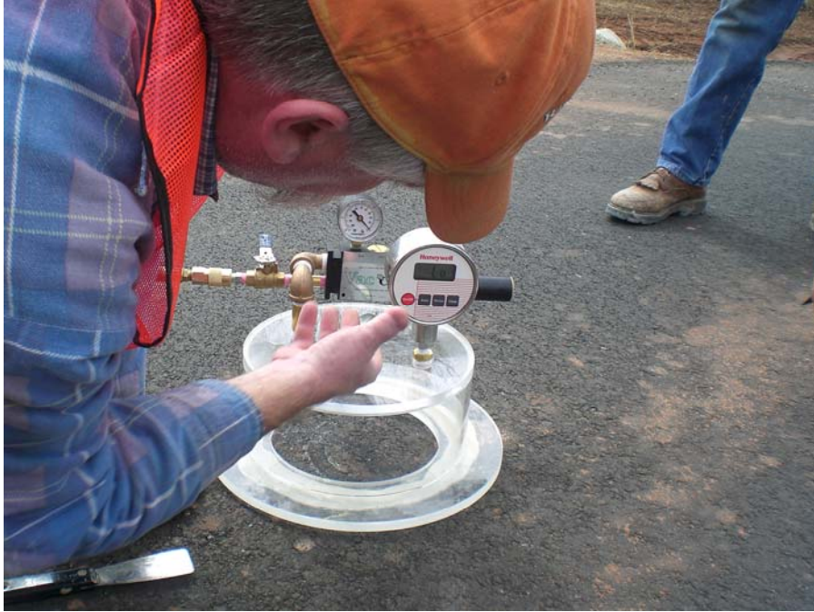
Figure 9 Measuring field permeability using the AIP.
