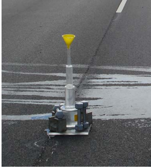
Figure 2 OSU's NCAT permeameter.
