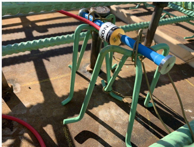
C. Concrete embedded strain gauge
