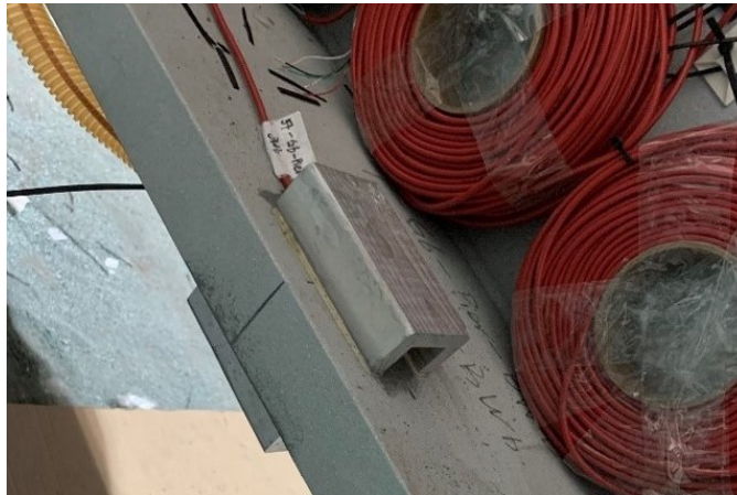
B. Weldable strain gauge (protected)
