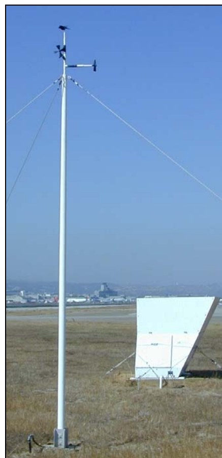
Figure 3-9. Sodar and 20-ft Anemometer Pole (beyond Runway 28L end of WL1)
