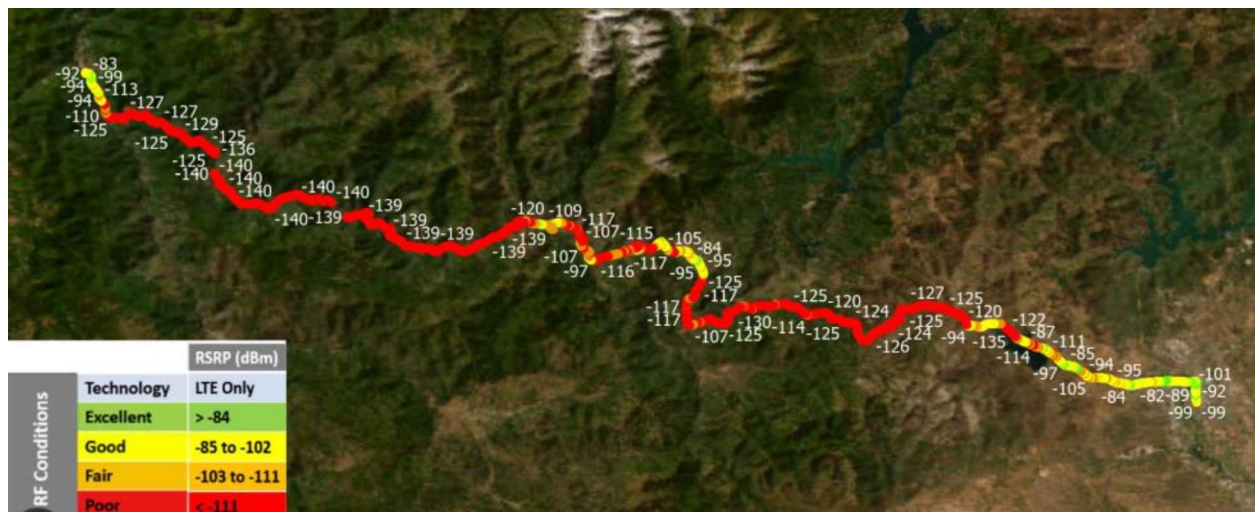
Figure A.3: Trial 1 – AT&T RSRP mapping result along Highway 299. Map generated using ArcGIS software by Esri.
