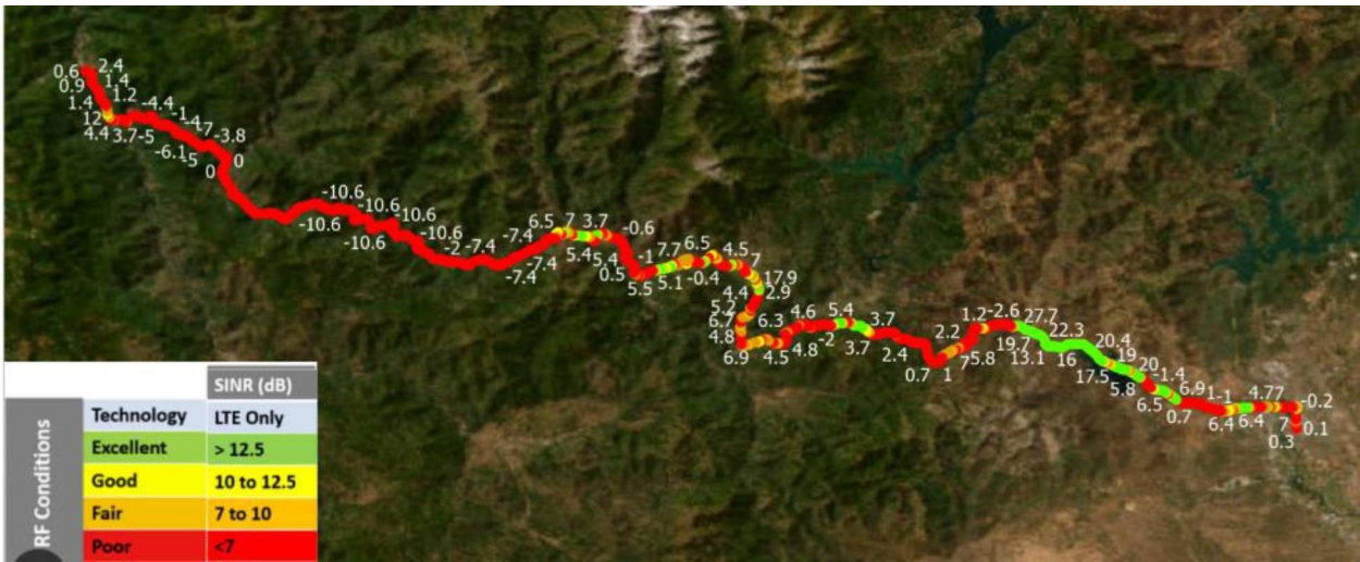
Figure A.12: Trial 1 – Verizon SINR mapping result along Highway 299. Map generated using ArcGIS software by Esri.
