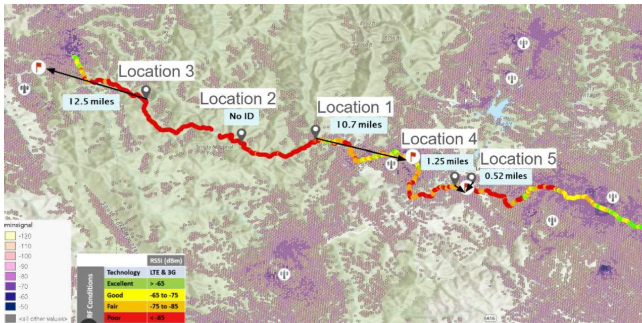
Figure 4.9: Highway 299 – Each location is mapped to its corresponding signal source, along with the distance from the location to the signal source. Map generated using ArcGIS software by Esri.
