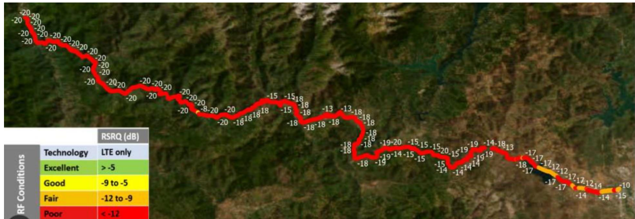
Figure A.14: Trial 2 – Verizon RSRQ mapping result along Highway 299. Map generated using ArcGIS software by Esri.
