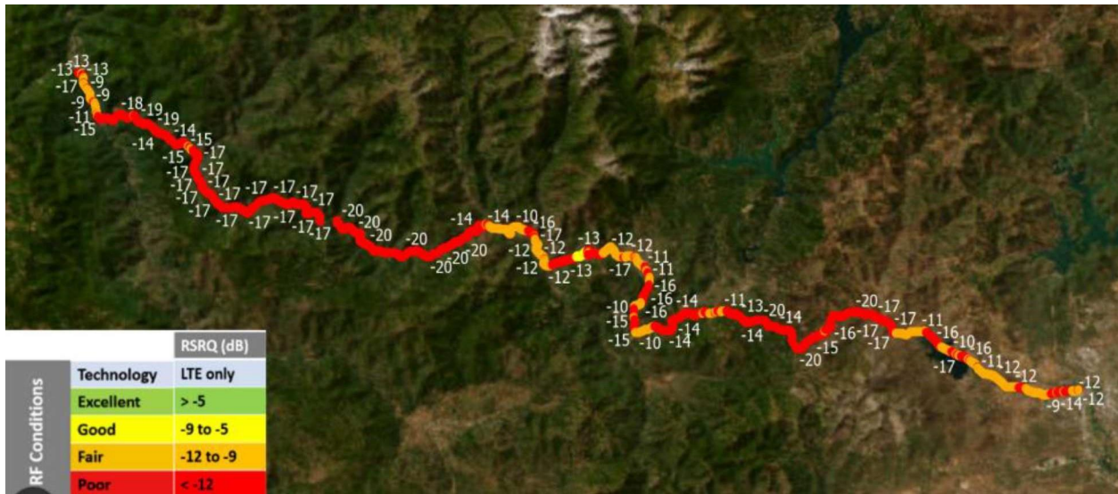
Figure 3.2: Trial 3 – AT&T RSRQ mapping result along Highway 299. Map generated using ArcGIS software by Esri.
