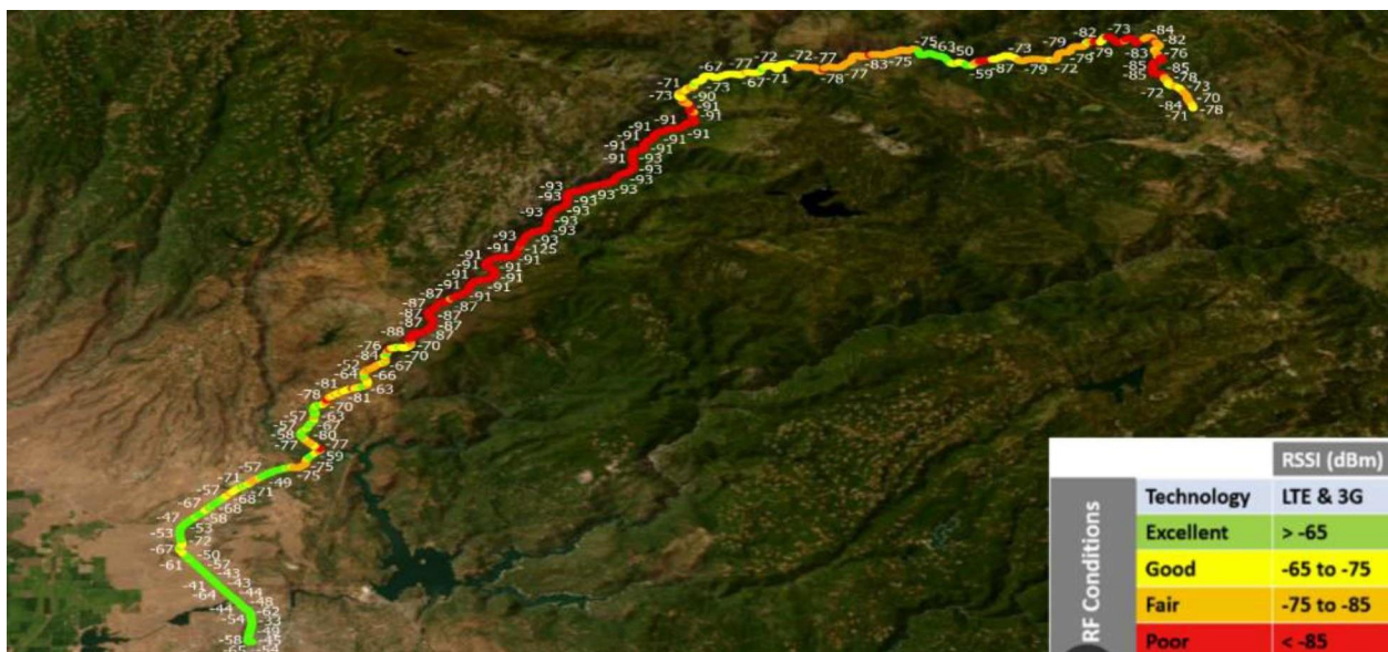
Figure 3.13: Trial 3 – Verizon RSSI mapping result along Highway 70. Map generated using ArcGIS software by Esri.
