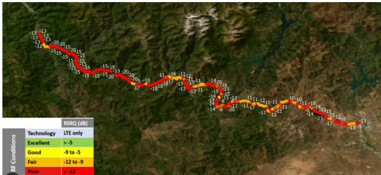
Figure 3.10: Trial 3 – Verizon RSRQ mapping result along Highway 299. Map generated using ArcGIS software by Esri.
