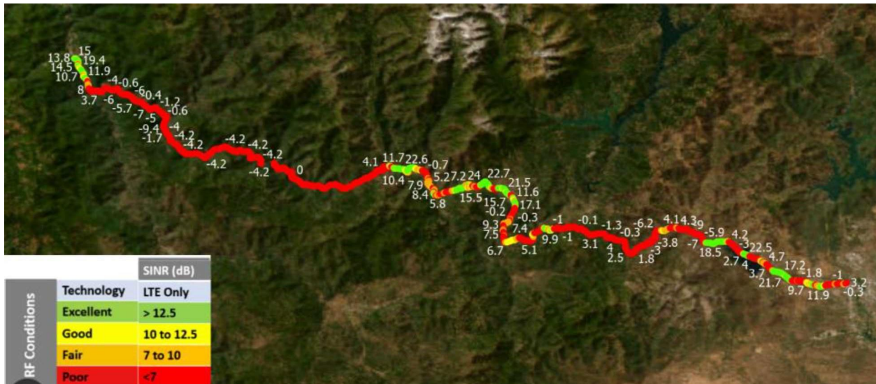
Figure 3.4: Trial 3 – AT&T SINR mapping result along Highway 299. Map generated using ArcGIS software by Esri.
