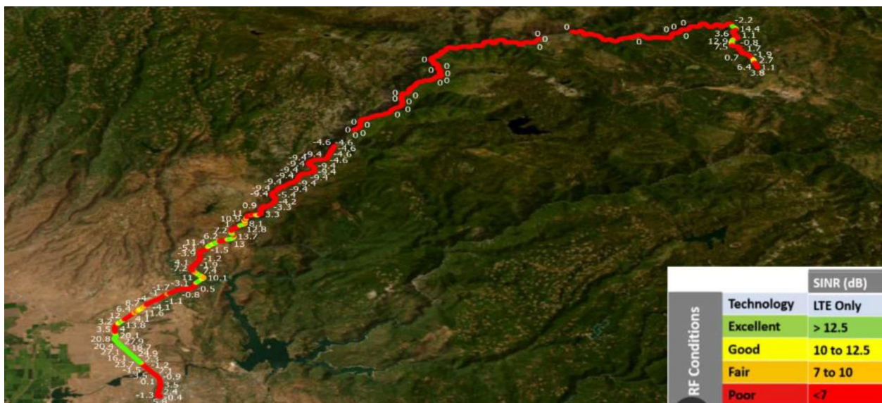
Figure 3.8: Trial 3 – AT&T SINR mapping result along Highway 70. Map generated using ArcGIS software by Esri.
