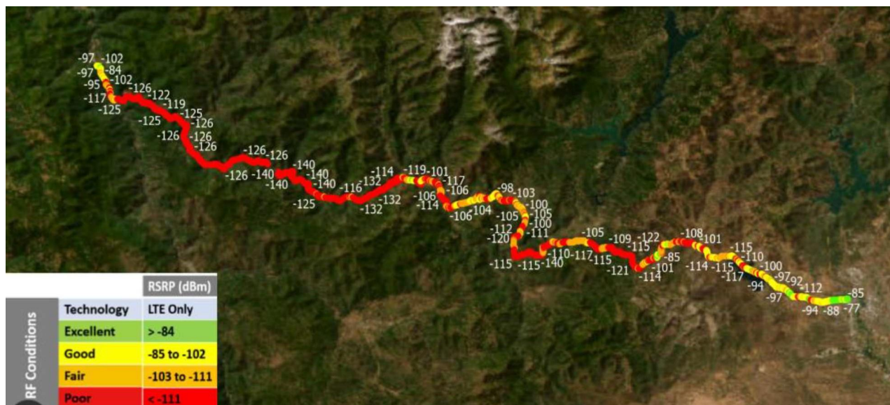
Figure 3.11: Trial 3 – Verizon RSRP mapping result along Highway 299. Map generated using ArcGIS software by Esri.
