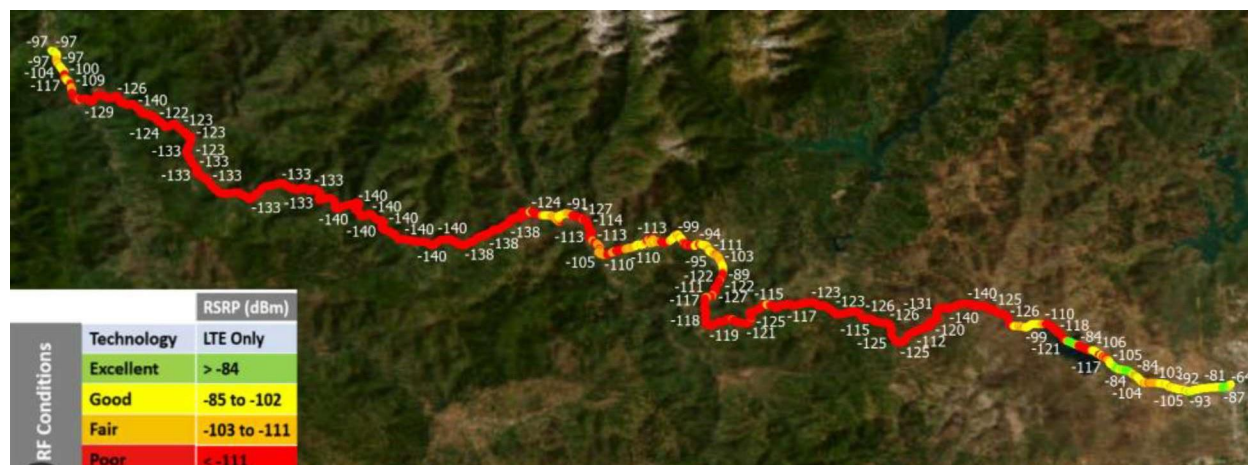
Figure A.7: Trial 2 – AT&T RSRP mapping result along Highway 299. Map generated using ArcGIS software by Esri.
