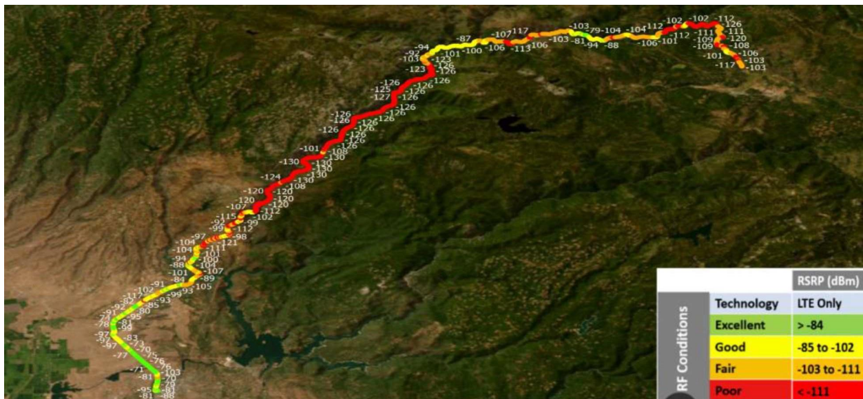
Figure 3.15: Trial 3 – Verizon RSRP mapping result along Highway 70. Map generated using ArcGIS software by Esri.
