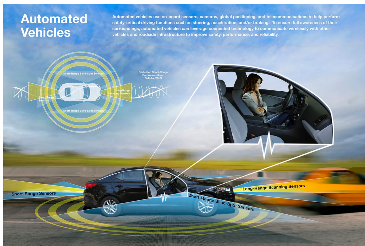
Graphic rendering of potential sensor placement on an automated vehicle
