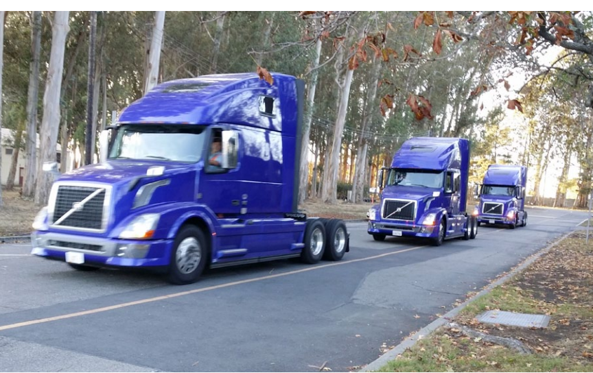
Test of truck platooning capabilities in California
