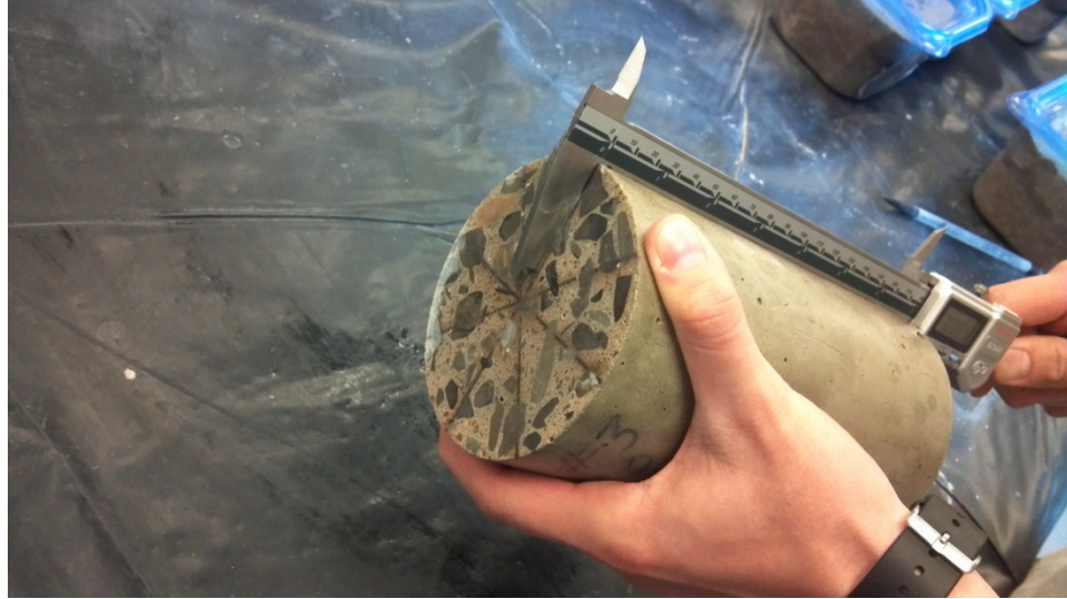
Figure 6.17 CTE cylinder during measurement with alignment markings
