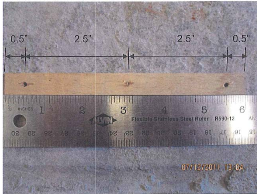
Figure 5.38 Laminated plywood dowel with dimensions
