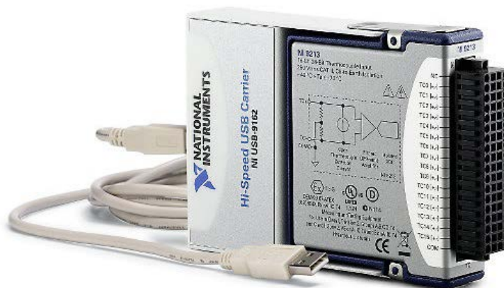
Figure 6.14 National Instruments USB signal carrier
