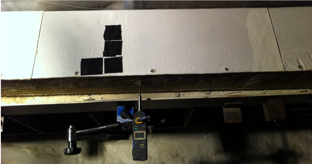
Figure 5.5 Plan view of the test setup showing the holes covered by tape, deflection gauge secured to the beam, and demec points glued on the surface of the concrete
