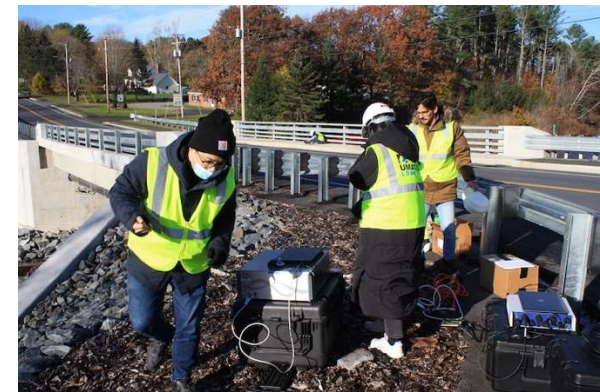
(a) Checking the condition of installed sensors. (b) Installation of an accelerometer on the bridge (c) Setup of optical sensor data collection system Figure 19. Preparation of field data collection at Grist Mill Bridge, Hampden, ME during November 3~4, 2021
