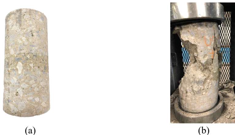
Figure C.7 Material property measurements: (a) field core, (b) after the compressive strength test.
