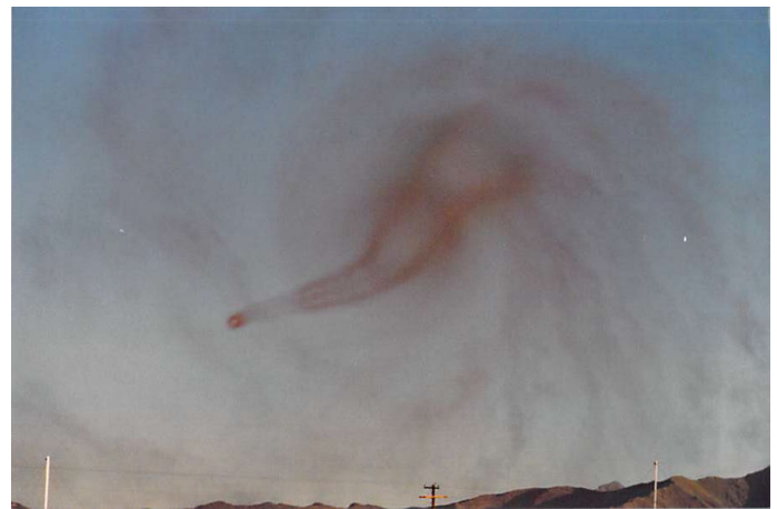
Smoke flow visualization of the vortex core conducted by the Federal Aviation Administration at Idaho Falls, Idaho, 1990 USDOT John A. Volpe National Transportation Systems Center Photographic Archive (Donation from David C. Burnham)
