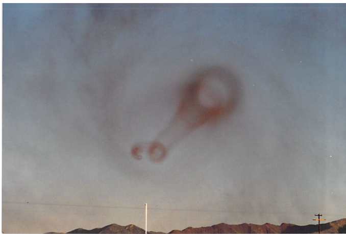
Smoke flow visualization of the vortex core conducted by the Federal Aviation Administration at Idaho Falls, Idaho, 1990 USDOT John A. Volpe National Transportation Systems Center Photographic Archive (Donation from David C. Burnham)
