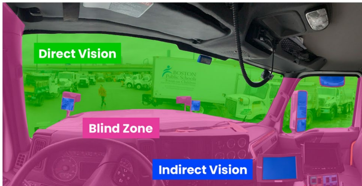
Figure 1: Driver's eye perspective of direct vision, areas visible through line of sight, indirect vision through mirrors and cameras, and the blind zone.
