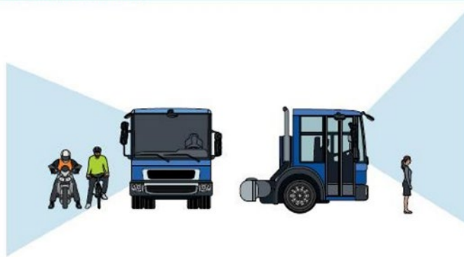
Figure 2. High vision and limited direct vision truck comparison.
