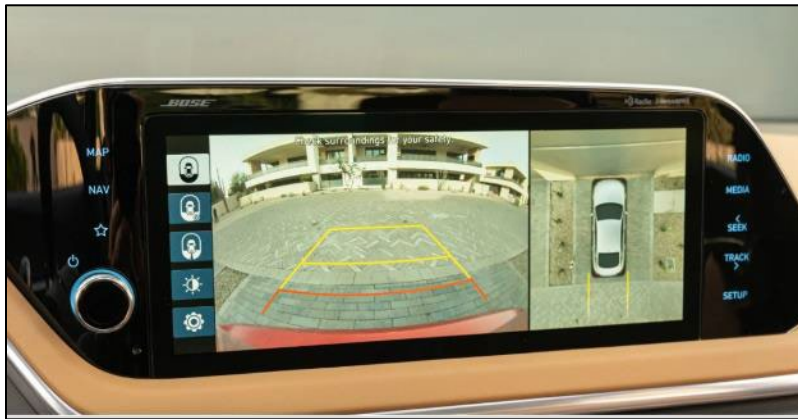
Figure 4. Split screen 360-degree camera and perspective view (OEM example)
