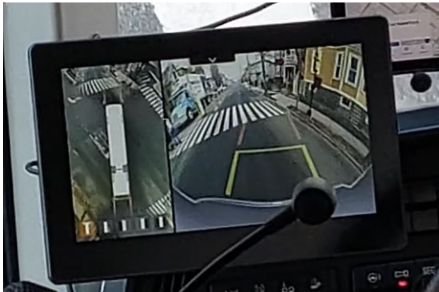
Figure 9: Split screen 360-degree camera and forward view (aftermarket example)
