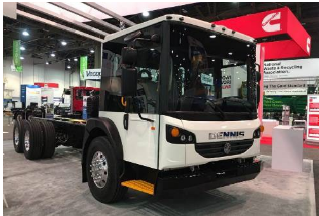
Figure 13: Example of available high vision cab model: Dennis Eagle Proview
