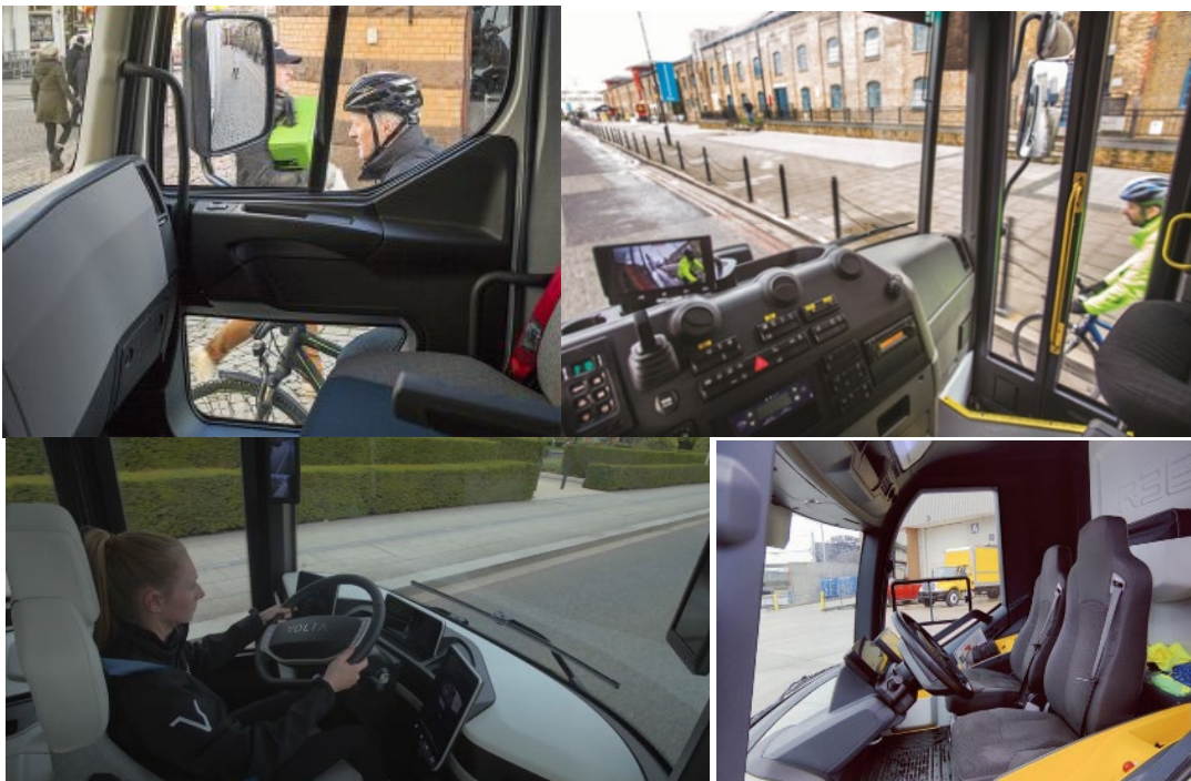
Figure 3: High-vision cabs expand near-vehicle visibility for drivers. Top: Mercedes/Freightliner Econic. Bottom left: Volta Zero. Bottom right: REE P7-C.
