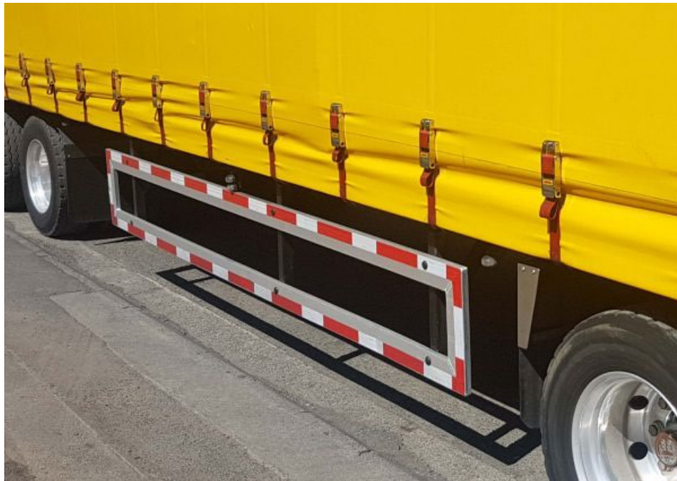
Figure 8. Lateral Protective Side Guard with Reflective Tape (Source: Right Driver) 34
