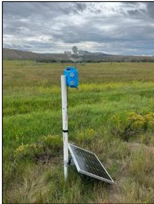
Figure 15. XPod Deployed at the US 40 Site with MET Station, Battery and Solar Panel
