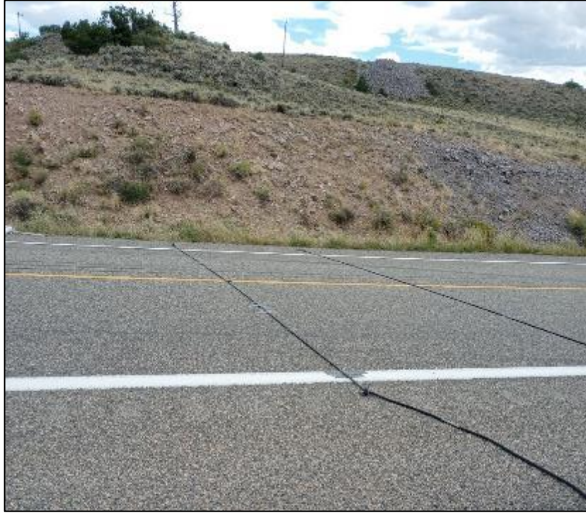
Figure 12. Pneumatic Road Tube Counters Placed Along US 50
