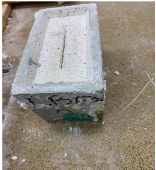
Figure 3.11b – MKP-VO cracked beam specimen
