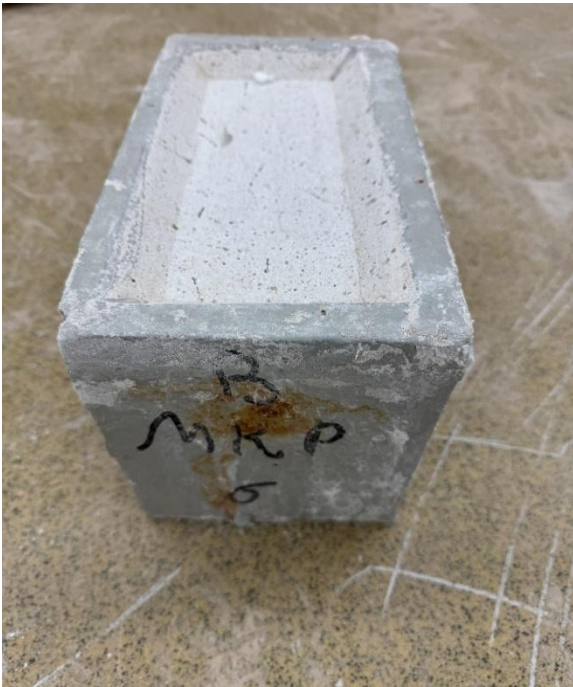
Figure 3.9a – MKP beam specimen
