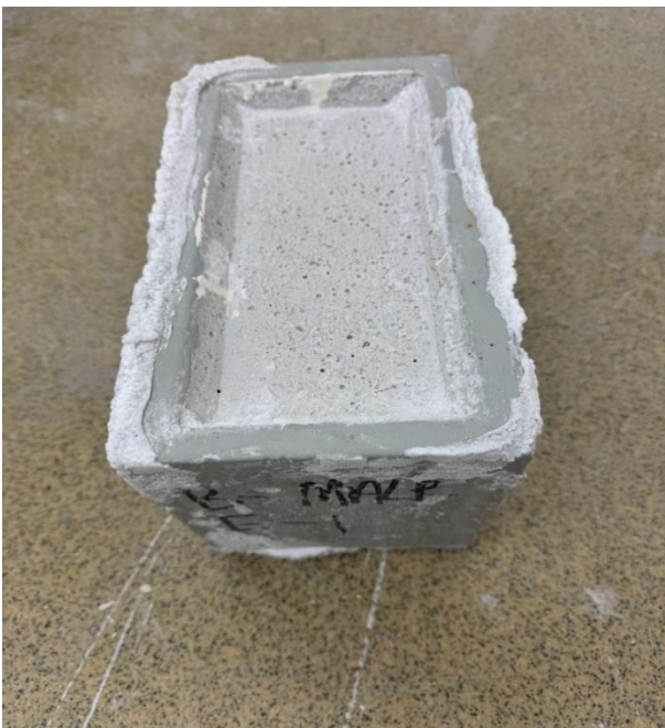
Figure 3.5a – MALP beam specimen with Endure (MALP-E)
