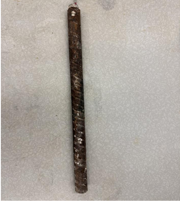
Figure 3.10a – Upper steel bar from MKP beam specimen
