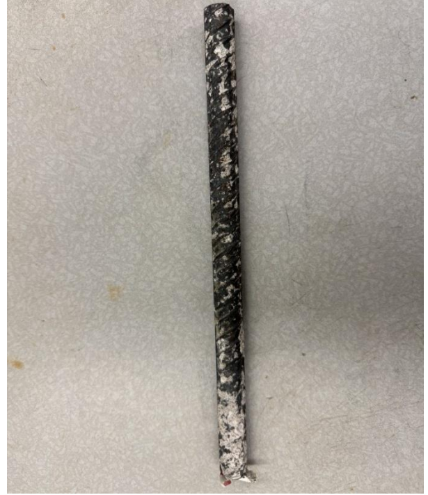
Figure 3.8b – Upper steel bar from MALP cracked beam specimens without Endure
