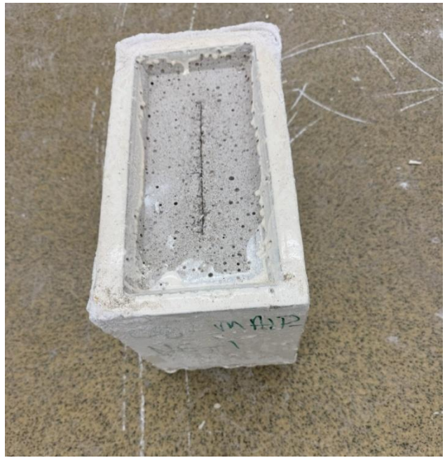
Figure 3.7b – MALP cracked beam specimen without Endure
