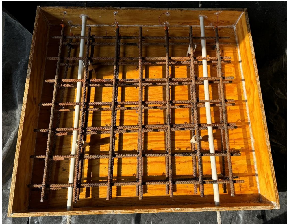
Figure 2.9: Form and reinforcing steel for field test specimen containing conventional concrete without MALP and without simulated cracks before casting
