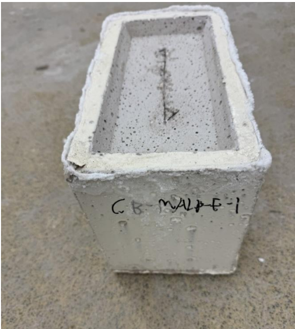
Figure 3.7a – MALP cracked beam specimen with Endure
