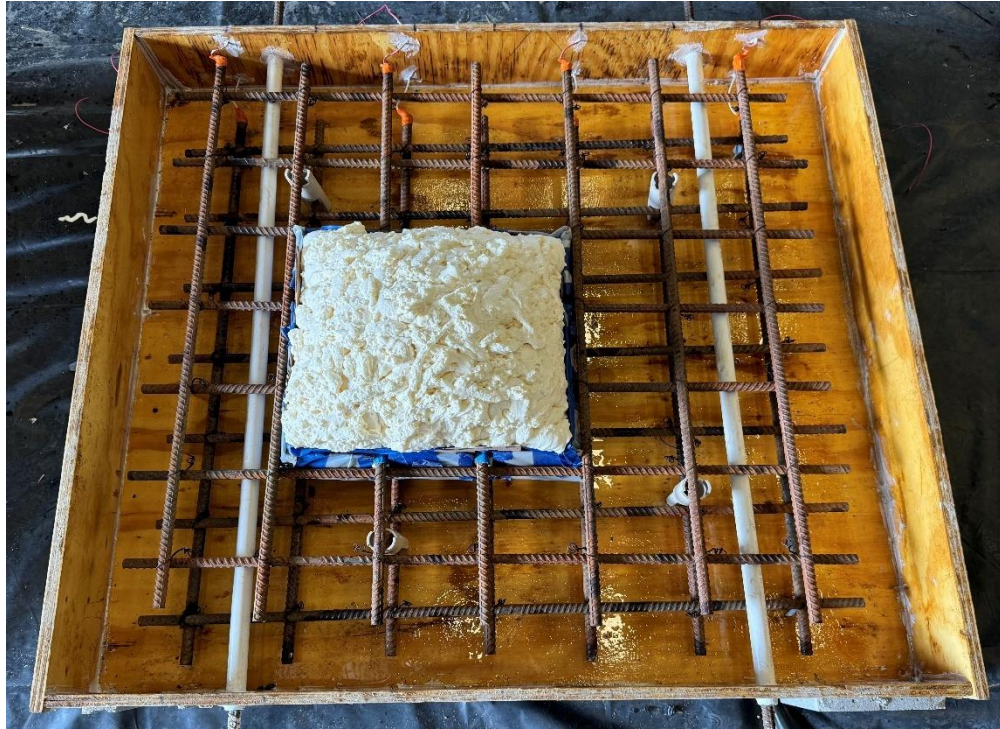
Figure 2.6: Form and reinforcing steel for MALP/Conv field test specimen showing the foam block-out used so that the edges of the repair patch aligned directly above the reinforcement (specimens with “A” in title) before casting
