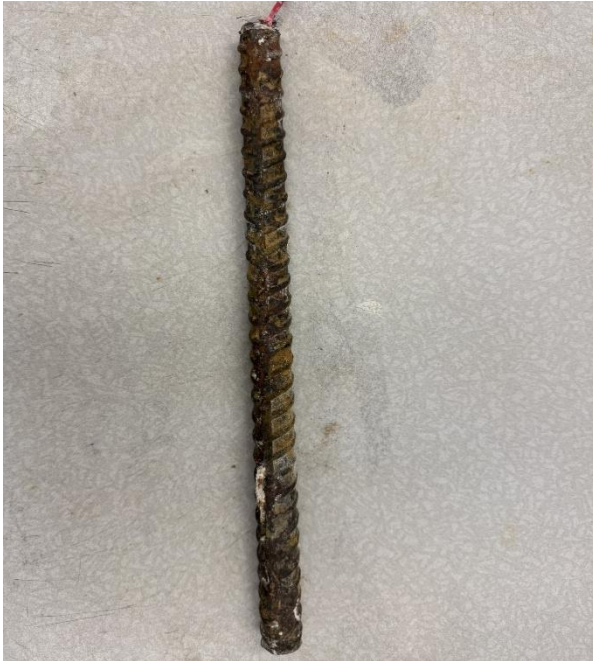
Figure 3.12a – Upper steel bar from MKP cracked beam specimen
