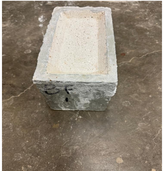
Figure 3.9b – MKP-VO beam specimen
