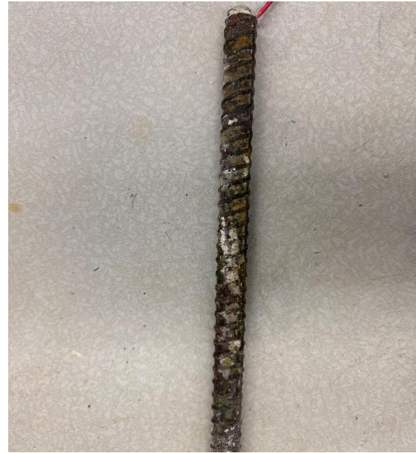
Figure 3.12b – Upper steel bar from MKP-VO cracked beam specimen
