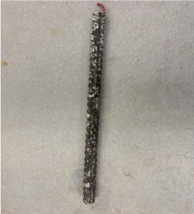
Figure 3.6a – Upper steel bar from MALP beam specimens with Endure
