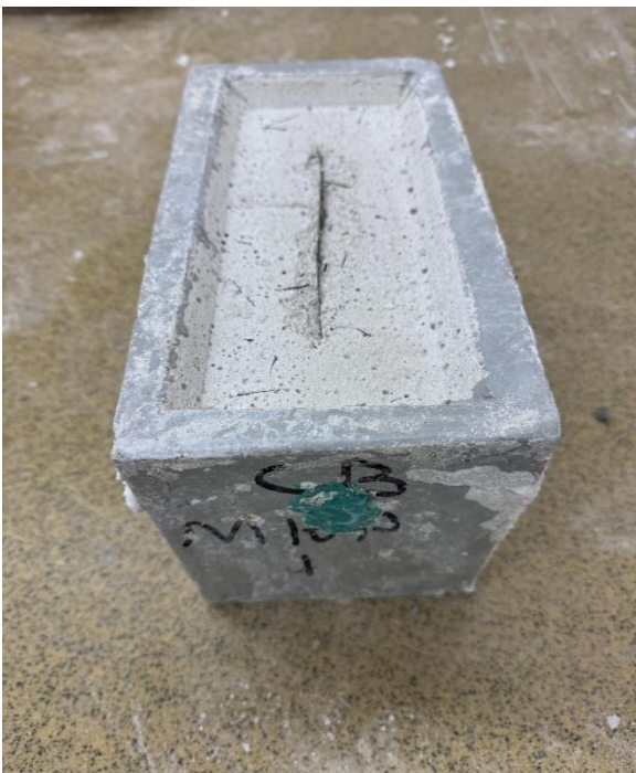
Figure 3.11a – MKP cracked beam specimen
