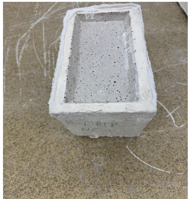
Figure 3.5b – MALP beam specimen without Endure (MALP-NE)
