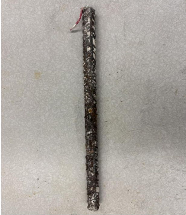
Figure 3.8a – Upper steel bar from MALP cracked beam specimens with Endure
