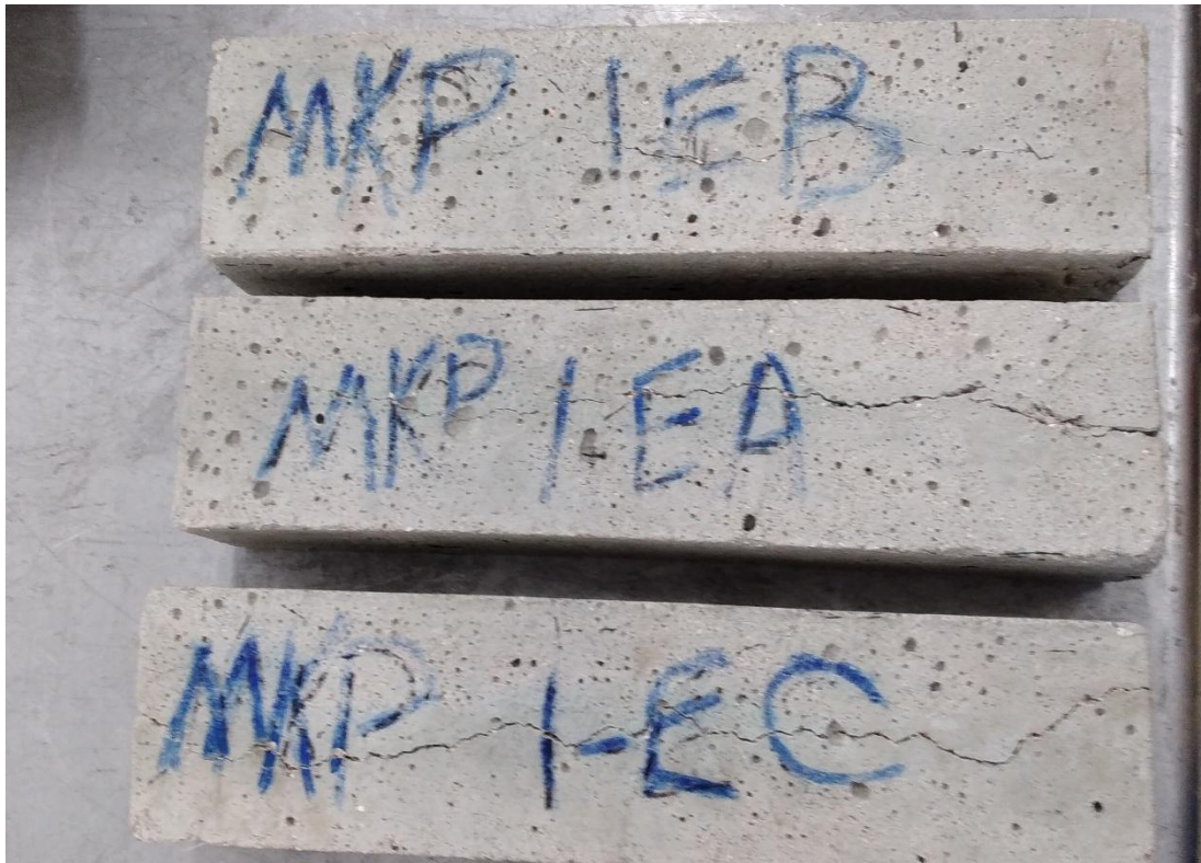
Figure 3.17- Three MKP specimens after 864 cycles (Procedure B) in freeze-thaw testing
