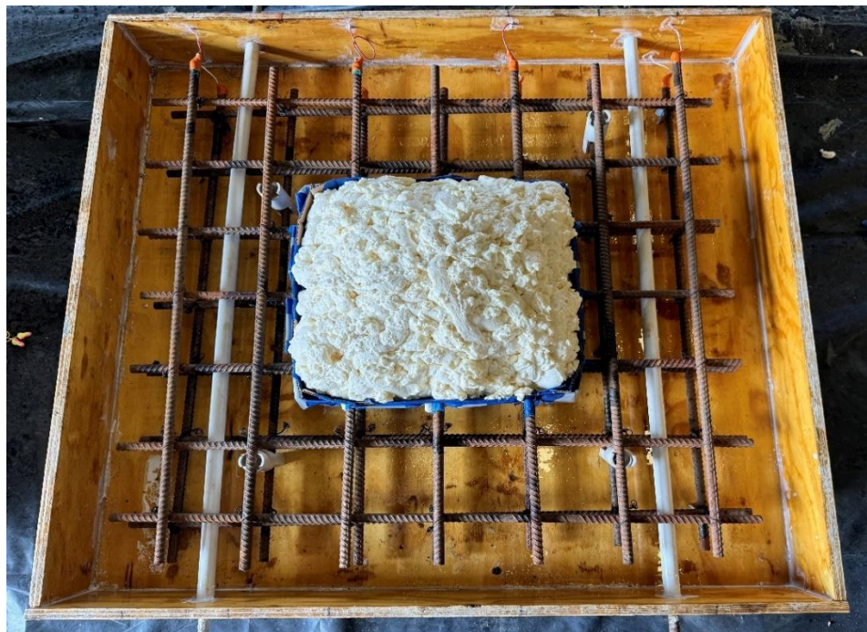
Figure 2.7: Form and reinforcing steel for MALP/Conv field test specimen showing the foam block-out used so that the edges of the repair patch aligned between reinforcing bars (specimens with “B” in title) before casting
