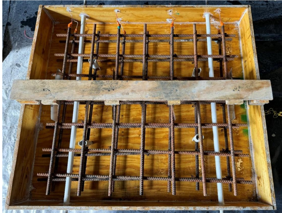
Figure 2.8: Form and reinforcing steel for field test specimen containing conventional concrete without MALP and with simulated cracks before casting
