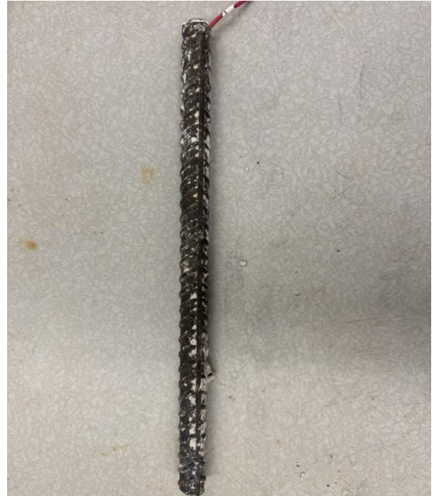
Figure 3.6b – Upper steel bar from MALP beam specimens without Endure
