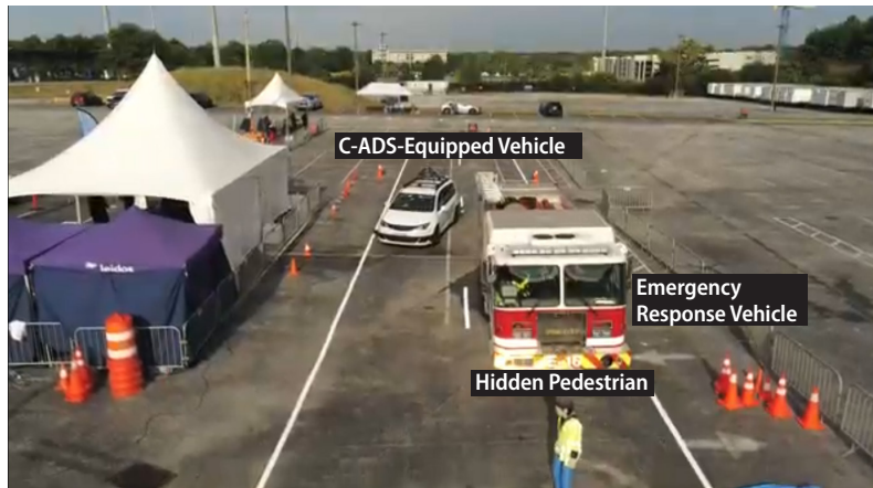
A. Infrastructure components detecting a hidden pedestrian crossing in front of an emergency response vehicle.
