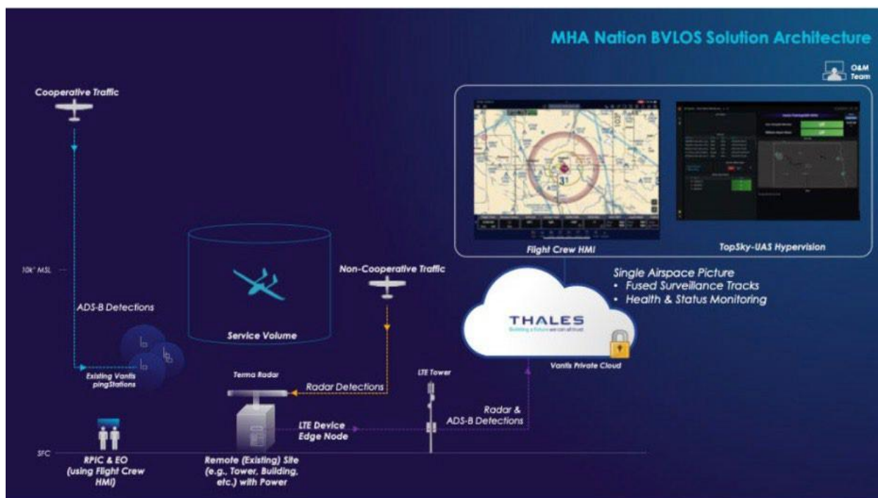
The Vantis System BVLOS Proposed Architecture with Ground Radar
