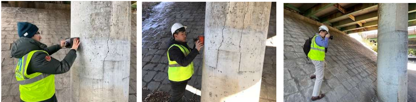
Figure 2. (a) GPR inspection of corroded RC bridge pier column (Koosha and Nak); (b) Visual inspection of RC bridge pier column (PI Yu)
