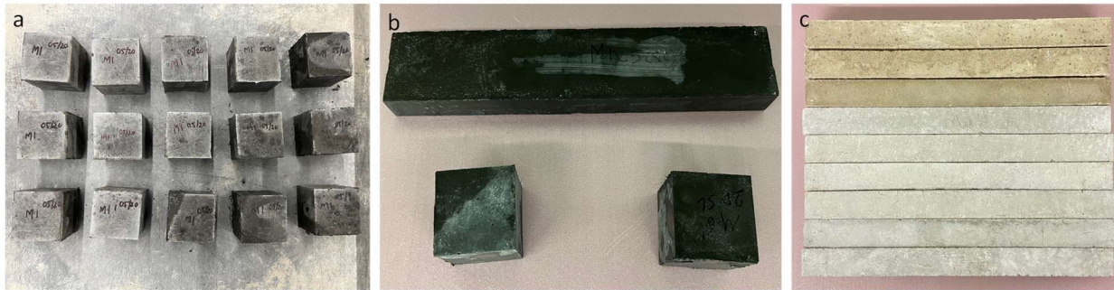
Figure 3. (a) cubes for compressive strength test, (b) beams for flexural strength test, and (c) mortar bars for ASR expansion test.
