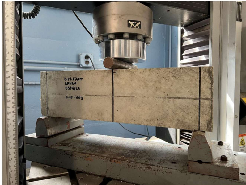
Figure 4. Flexure Test Setup (Three-Point)
