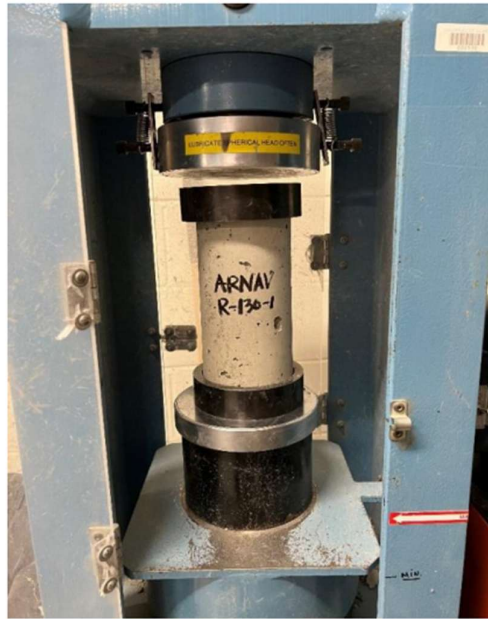
Figure 5. Compression Test Setup
