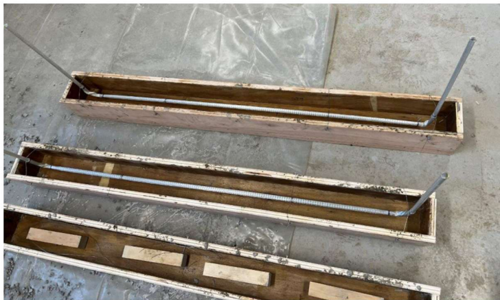
Figure 7. PETG Rebars Placed in Molds Prior to Casting
