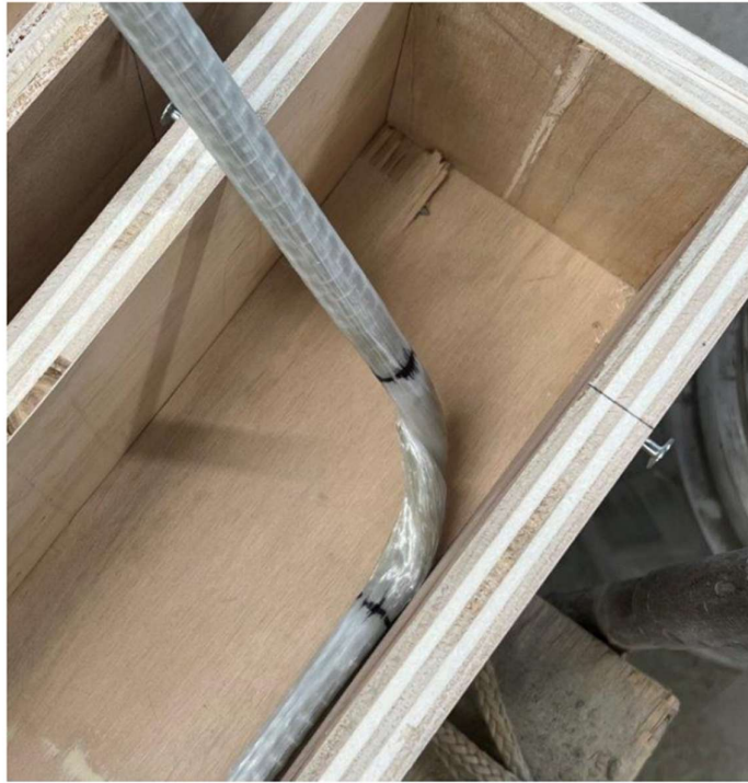
Figure 8. PETG Rebar Bend Profile
