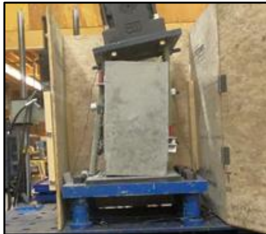
Figure 2-12: Shear Block 3 Premature Failure
