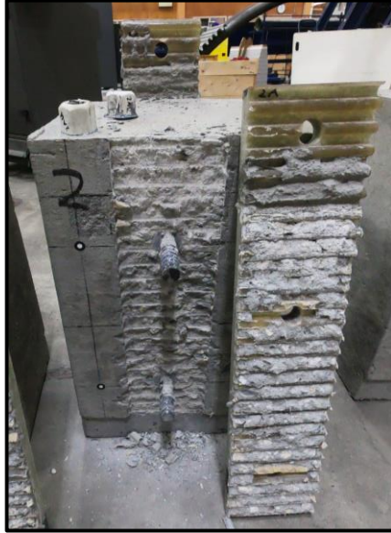
Figure 2-26: Shear Block 2 Failure
