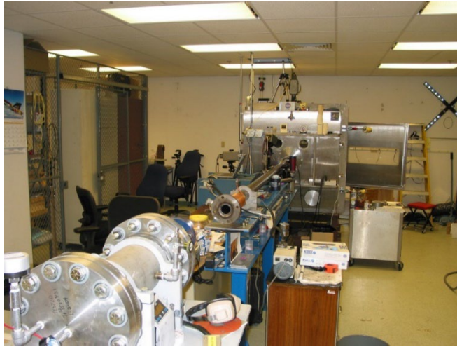
Figure 24. Single stage gas gun setup at NASA Glenn Research Center
