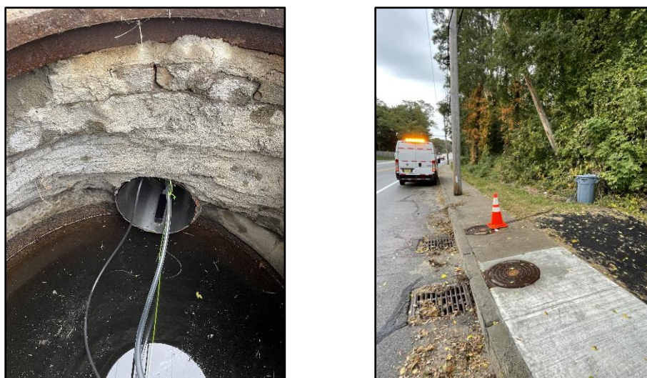
Figure 3-4: Autosampler setup for stormwater sample collection.
