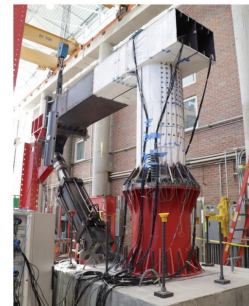
Figure 3.63: Knee joint test setup for Test 2 specimen (D1 = 44).
