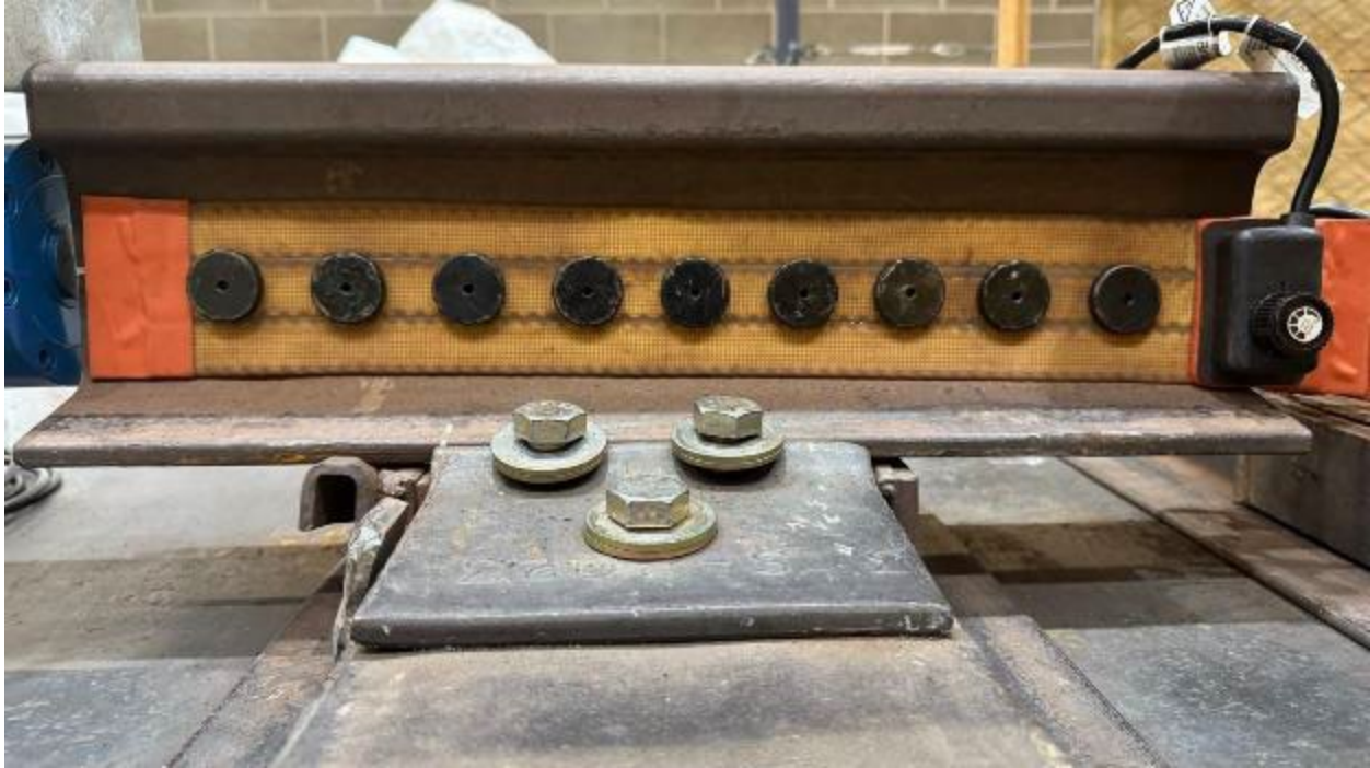
Figure 6. Side view of the rail with heating tape secured by magnets.
