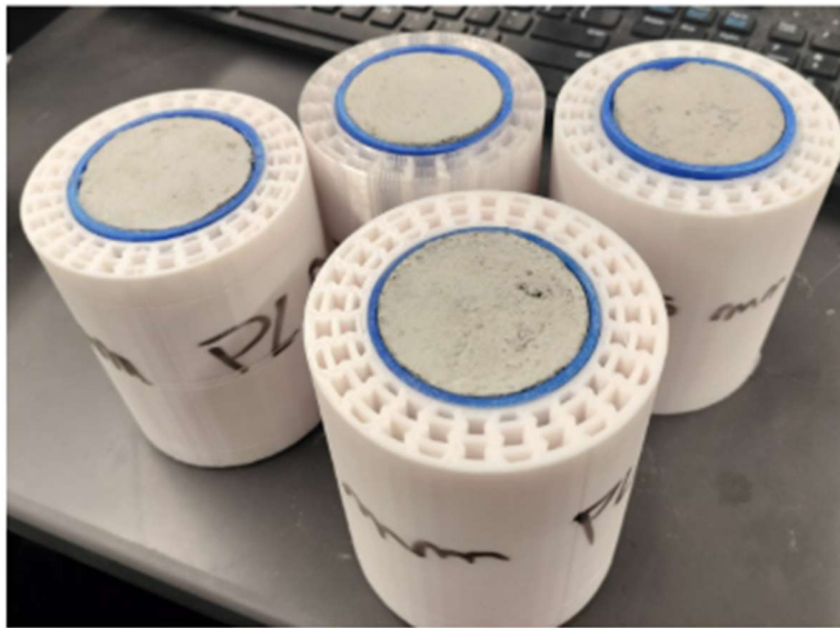
Fig. 3 — Representative re-entrant auxetic cores and integration around mortar cylinders
