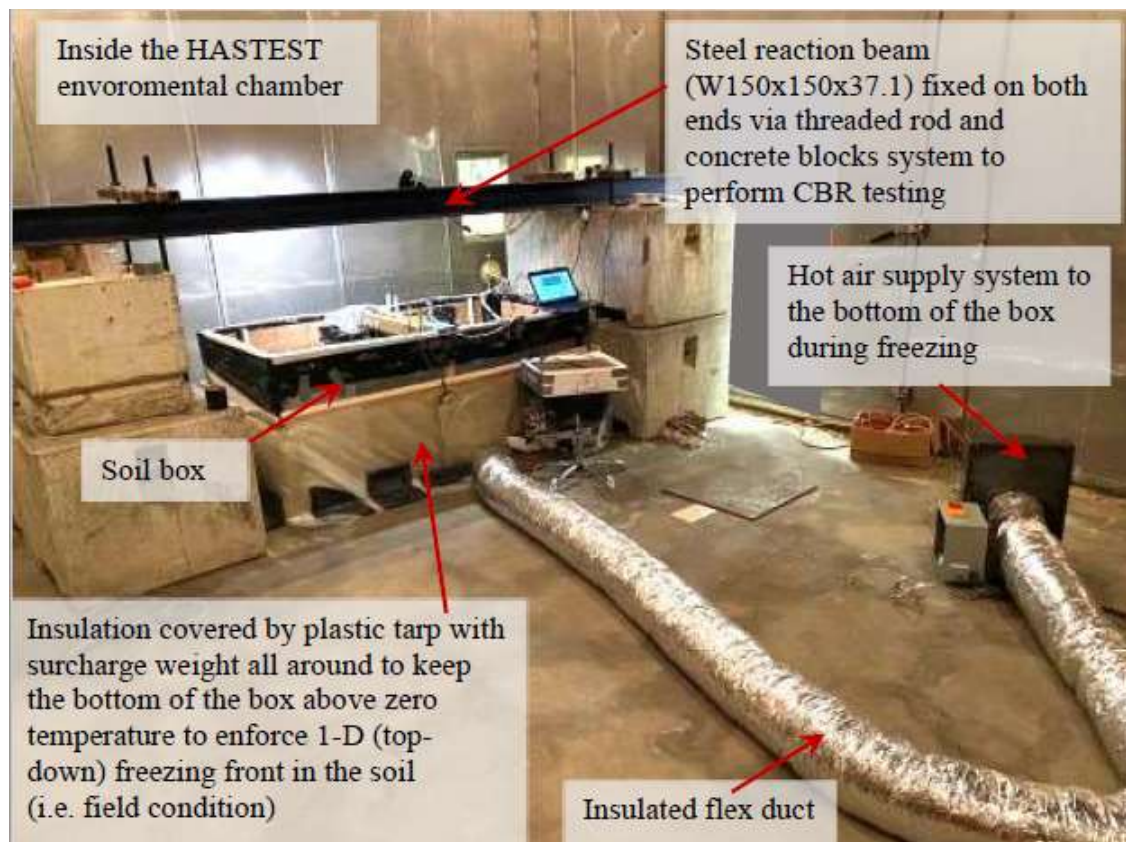
Figure 24. Overview of experimental setup and equipment used for the large-scale freeze-thaw experiments in the HASTEST environmental chamber, including insulation and heating system used to heat underside of the box and the beam and reaction blocks used for field CBR testing at different stages of testing.
